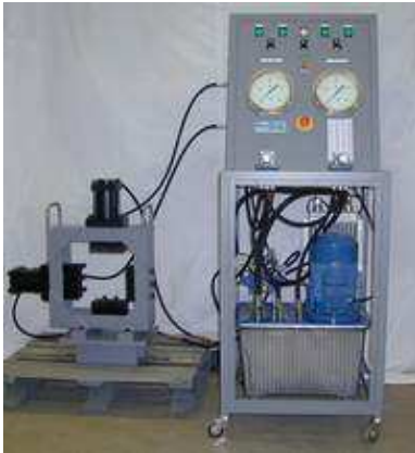
Fig.10. Biaxial preload device
