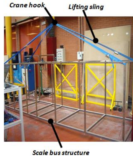
Figure 10. Scale bus structure hanged from a bridge crane.
