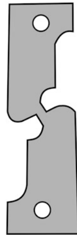
Fig. 17 Types of specimens for dynamic punch tests. Modification of the radius R_n of circular notch allows to obtain different values of the triaxiality and the Lode parameter
