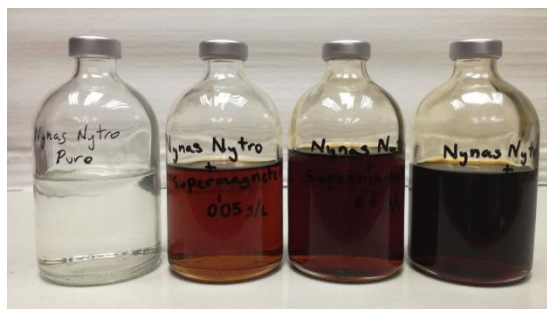
Figure 1: Oil samples with different concentrations of NP. From left to right: 0 g / L, 0.05 g / L, 0.1 g / L and 0.2 g / L.
