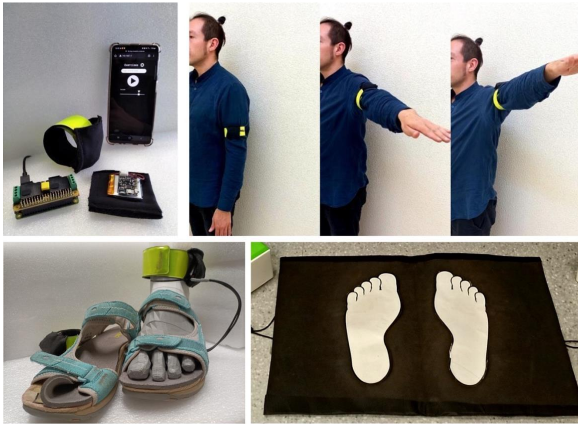
Figure 2: Technological Probes brought to the workshop. Top left: Soniband is a wearable band that integrates a BITalino R-IoT embedding a 9-axis Inertial Motion Unit (IMU). The R-IoT transmits movement angle data wirelessly to a Raspberry Pi Zero, which can be controlled using a web browser in e.g., a smartphone. The device registers the minimum and maximum angle of the body part (calibration), and then it sonifies movement angle real-time with five movement-sounds: “Wind”, “Water”, “Mechanical”, “Ascending Tone” and “Beep.” (see more details in [21]). In the workshop, the participants could choose the movement to sonify and the sound. Further details can be found in [21]. Top right: Example of movement sonified by Soniband. Bottom left: Sonishoes integrate a Soniband worn in the ankle and a sole that detects pressure against the ground and “sonifies” steps. Sonishoes allowed five different movement-sound conditions: “Aluminum can crush” (replicating the sense of pressing a coke can against the ground), “Wind” (a pink noise sound changing frequency which plays during the foot swing of a stride or in response to changes in leg angle), “Water” (a continuous sound of water running with a “splash” sound at certain angle), “Mechanical” (a gears sound changing with angle), and “Tone” (a continuous tone plays from start to end of the movement). Further details can be found in [20]. Bottom right: Sonicarpet is a simpler version of Sonishoes, which just sonifies steps when stepping on it (i.e., when detecting pressure against the ground).
