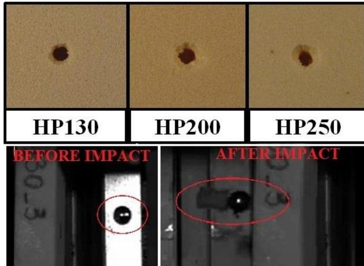
**Figure 6:** Plugging damage mode typical of PVC foams and 110 m/s impact progression of a HP130 foam
