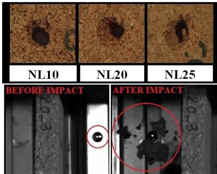
**Figure 7:** Conical intergranular fracture typical of agglomerated corks and 84 m/s impact progression of a NL20 agglomerated cork
