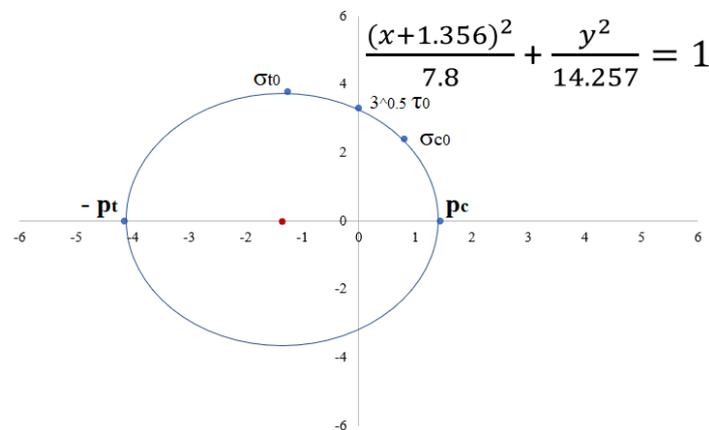
**Figure 3:** Yield surface of HP130 employed to calculate  $p_t$  and  $p_c$
