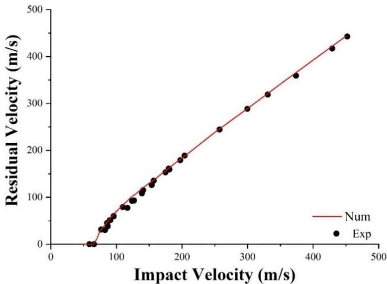
**Figure 10:** Fitting between the experimental data and the numerical simulation of HP130 PVC foam
