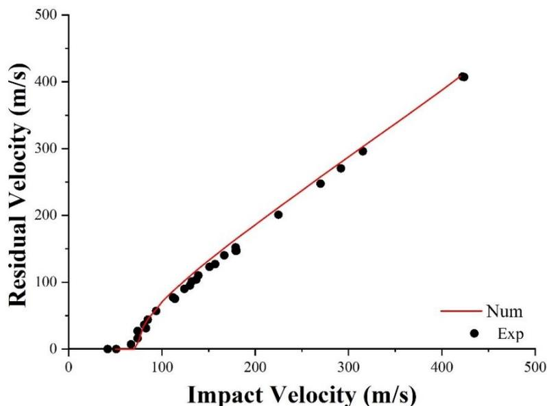
**Figure 11:** Fitting between the experimental data and the numerical simulation of NL25 agglomerated cork
