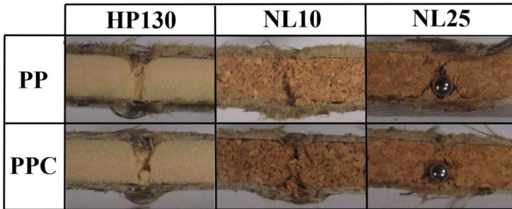
**Figure 9:** Cross-sections of the six sandwich configurations impacted at 175 m/s which allowed to estimate the damage experienced by the composites
