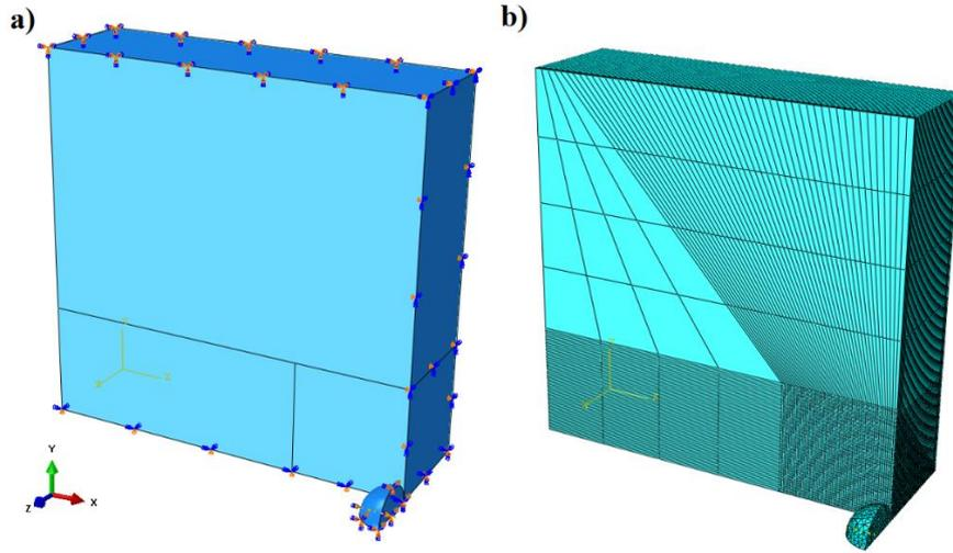
**Figure 2:** Quarter model employed to carry out the finite element analysis: boundary conditions (a) and mesh distribution (b)
