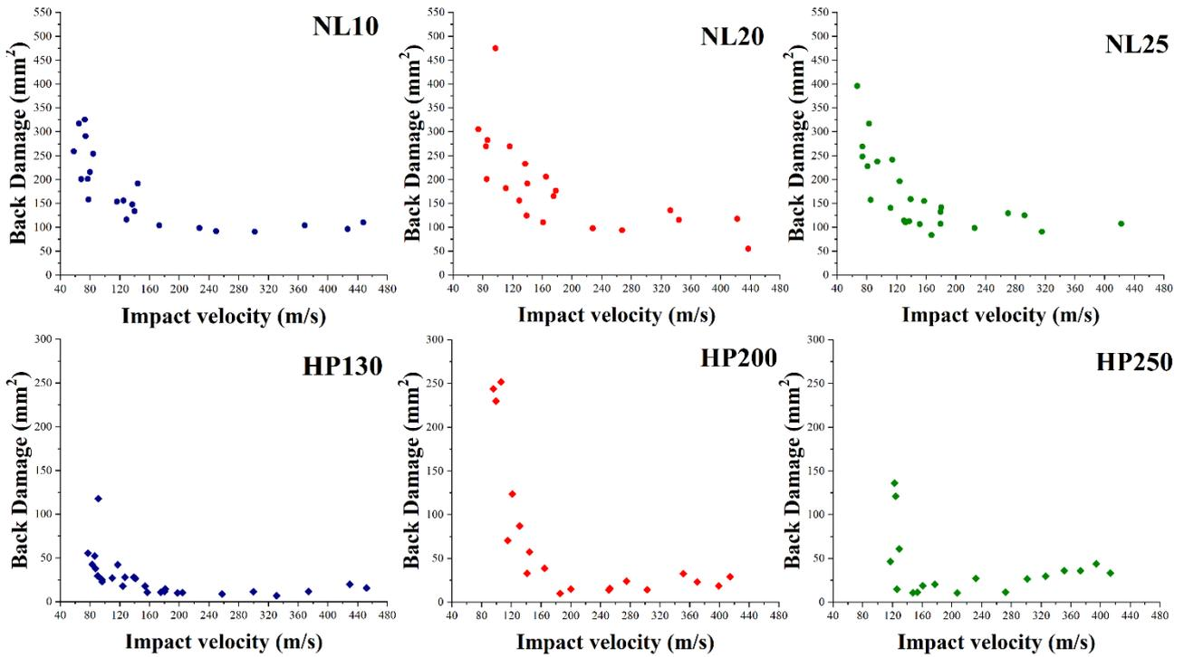
**Figure 8:** Evolution of back damage area extent as a function of impact velocity for the six core materials
