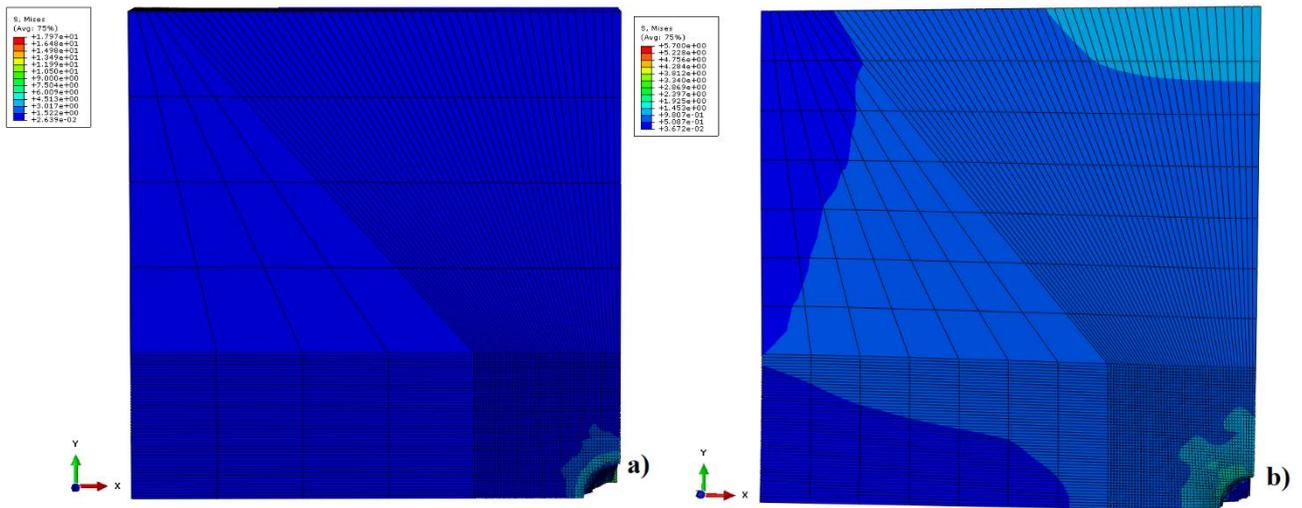
**Figure 12:** Von Mises stress distributions for HP130 (a) and NL25 (b)
