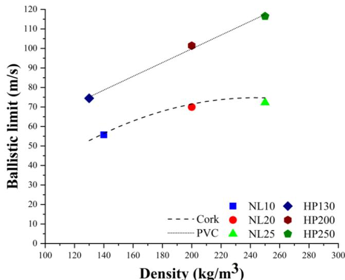
**Figure 5:** Ballistic limits of the six core materials calculated through the Lambert-Jonas equation as a function of core density
