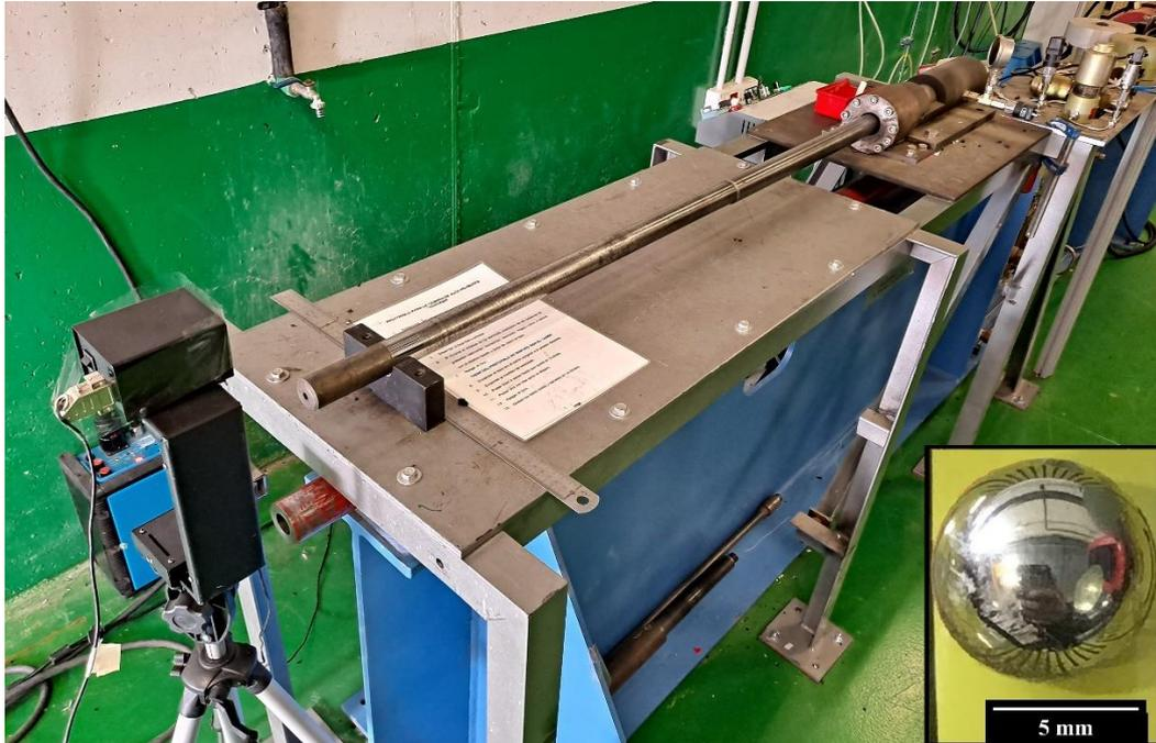
**Figure 1:** Gas gun and projectile used to perform ballistic impact tests
