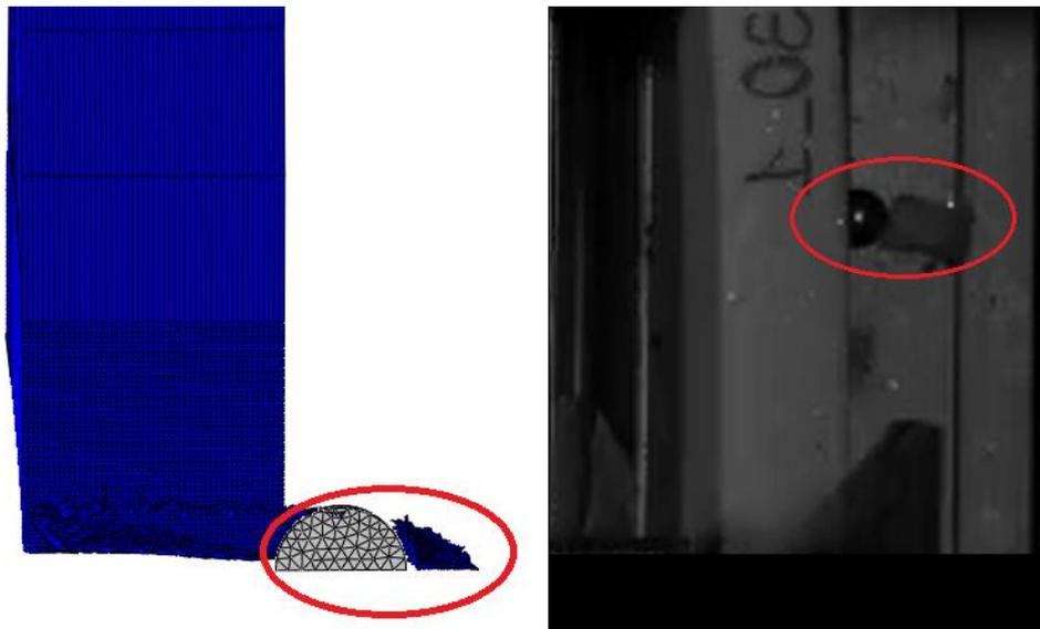
**Figure 13:** HP130 damage mode numerical v.s. experimental
