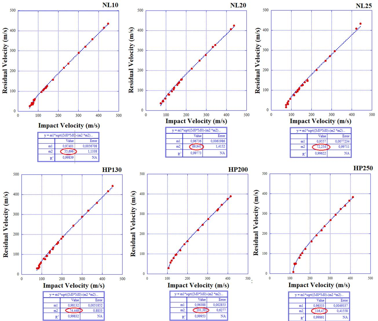
**Figure 4:** Agglomerated cork (NL10, NL20 and NL25) and PVC foams (HP130, HP200 and HP250) experimental data (red dots) and interpolation curves (blue line) obtained implementing the Lambert-Jonas equation through a least square method
