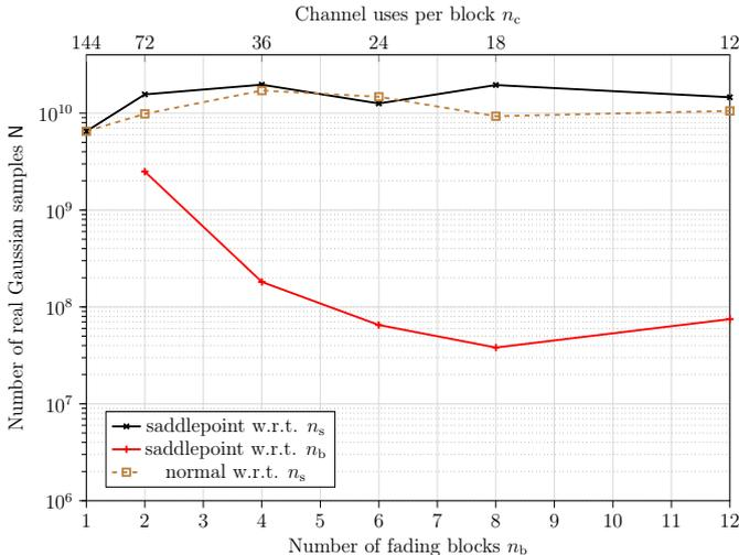
Fig. 7: Two-user, single-cell massive MIMO scenario: required number of real Gaussian samples to guarantee that  $e(N) \leq 0.5\%$ . Here,  $n_b n_c = 144$ ,  $R = 2$  bit per channel use,  $n_p = 2$ ,  $N_{\text{sim}} = 100$ , and  $\epsilon = 10^{-5}$ .
