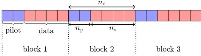
Fig. 1: Structure of a packet for  $n_c = 6$ ,  $n_p = 2$ ,  $n_b = 3$ .
