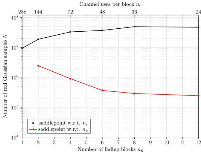
Fig. 5: Required number of real Gaussian samples to guarantee that  $e(N) \leq 0.5\%$ . Here  $n_b n_c = 288$ ,  $R = 0.104$  bit per channel use,  $N_{\text{sim}} = 100$ , and  $\epsilon = 10^{-5}$ .
