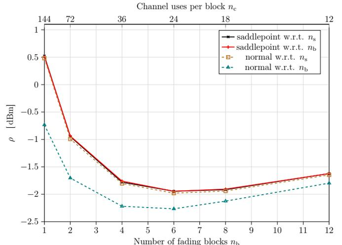
Fig. 6: Two-user, single-cell massive MIMO scenario: required transmit power  $\rho$  to achieve  $\epsilon = 10^{-5}$ . Here,  $n_b n_c = 144$ ,  $R = 2$  bit per channel use, and  $n_p = 2$ .
