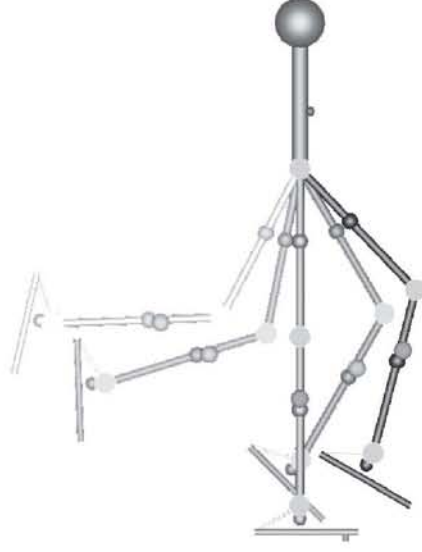
Figure 5.7: Stroboscopic animation of the “kicking” experiment. This experiment will compensate the torques produced by the inertia of the swinging leg. The objective is to demonstrate how precise is the four point model proposed in this chapter.
