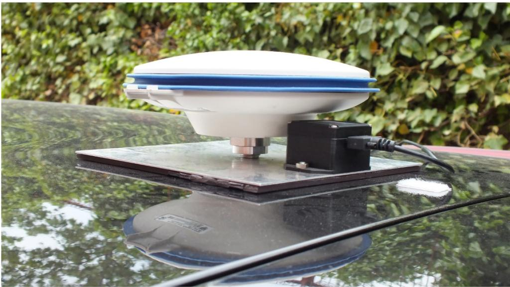
Figure 5.2: Mid-cost sensors as mounted in the roof of the test vehicle.
