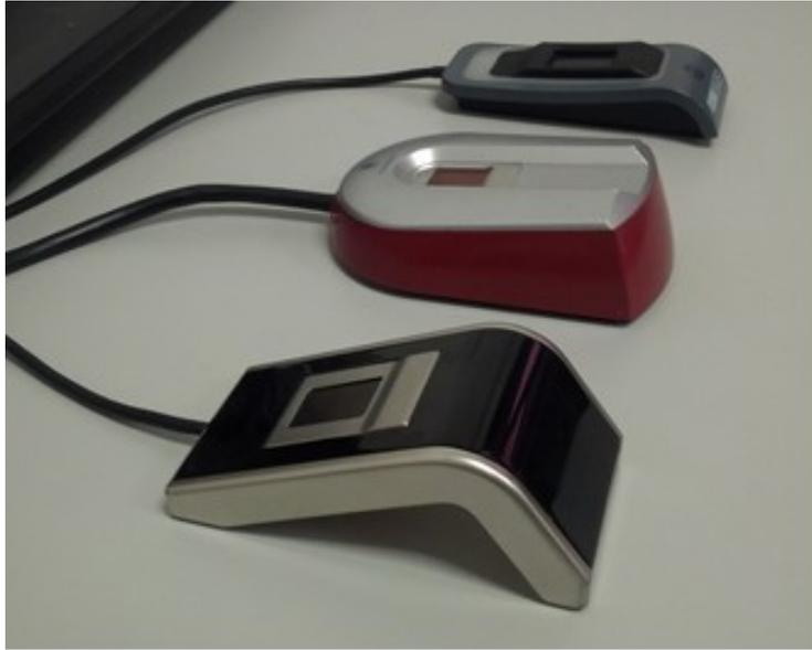
**Figure 47. Fingerprint sensors used in the experiment. From bottom to top: NEXT, Fingerprints and Upek**
