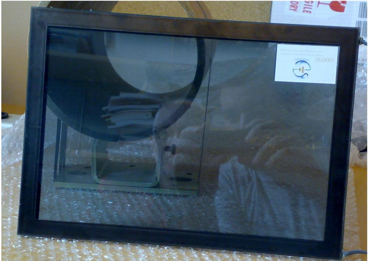
Figure 2: Photograph of the SPD sample for dark and bleached states.
