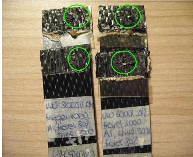
Figure 31. Broken fibers in one of the side of the welded area
