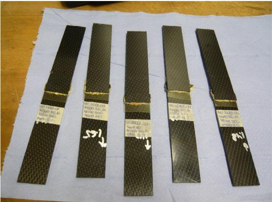
Figure 23. Samples after welding
