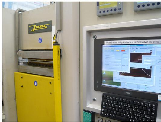
*Figure 12. Press to make the laminates*
