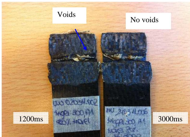
Figure 29. Difference between solidification time 1200ms and 3000ms
