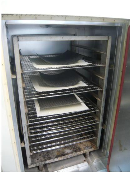
*Figure 11. Oven to dry the layers of CF-PEI*
