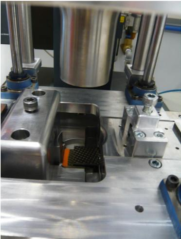
Figure 21. Samples ready to be welded
