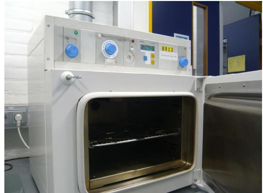
*Figure 15. Oven to remove the moisture of the samples*
