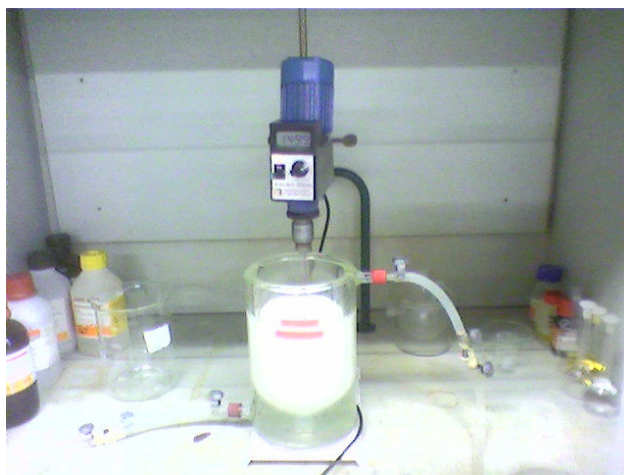
Figure 3.2 Paddle stirrer and double wall beaker used during dichloromethane evaporation
