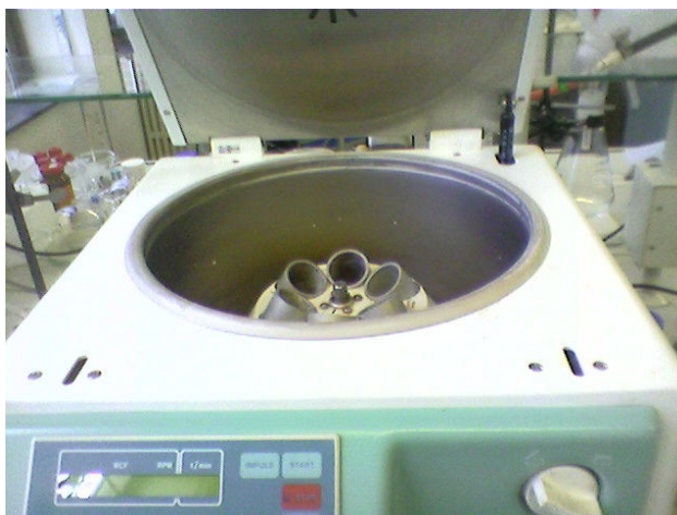
Figure 3.4 Centrifugation machine used for particles settling
