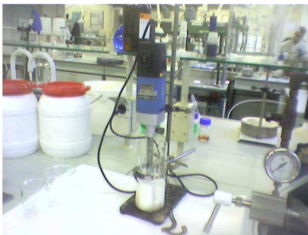
Figure 3.1 Ultra-Turrax used during microcapsules and solid polystyrene particles emulsification
