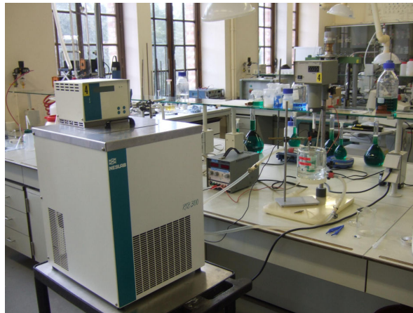
Figure 3.9 Rotating machine, current source and thermostatic bath
