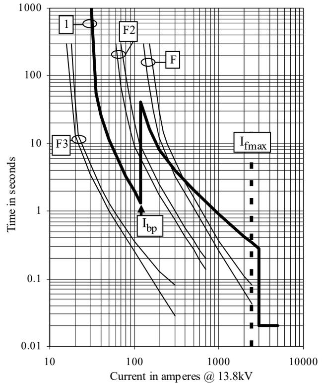
Fig. 10. Case of Fig. 3, considering 3 different downstream fuses and the afore-described nontraditional curves for the 51N function.
