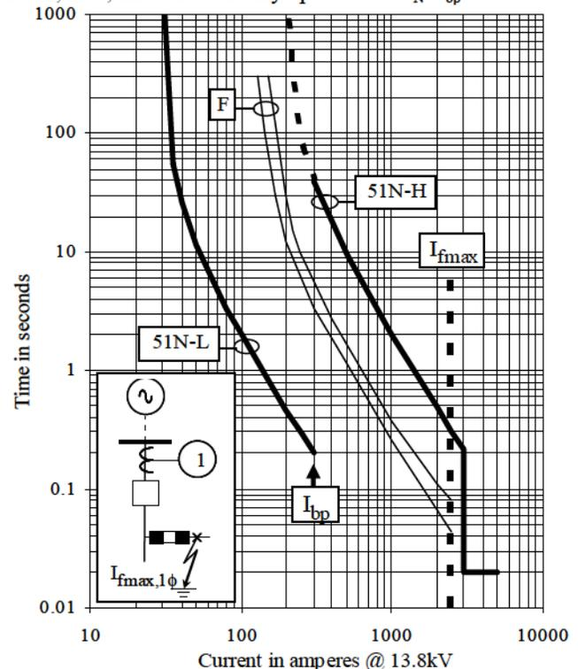
Fig. 5. Case of Fig. 3, implemented by applying logical combination of traditional curves (51N-L and 51N-H are 51N functions of relay 1).
