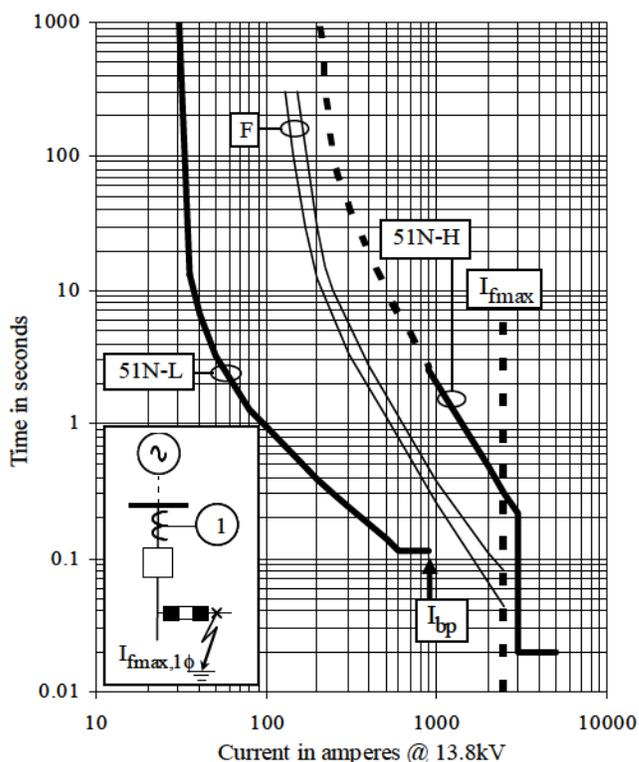
Fig. 8. Case of Fig. 4, implemented by applying logical combination of traditional curves (limits in curve shapes for  $M \geq 20$  are considered).
