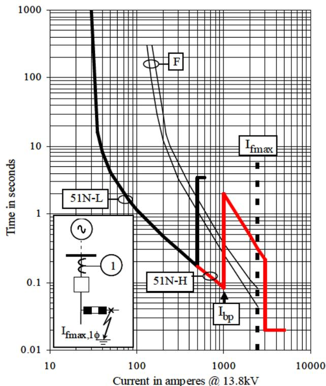
Fig. 7. Case of Fig. 4, implemented by applying curve shapes created by the user (limits in curve shapes for  $M \geq 20$  are considered).
