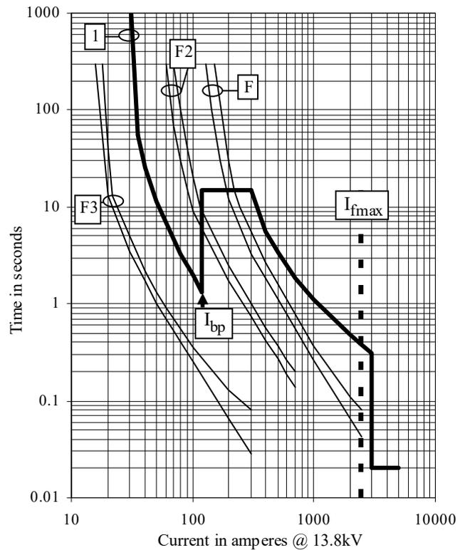
Fig. 11. Case of Fig. 3, considering 3 different downstream fuses and a different nontraditional curve (51N), in order to maximize selectivity.
