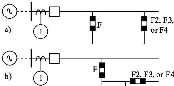
Fig. 9. Examples of configurations with downstream fuses: a) F2, F3 or F4 are in a different branch than F; b) F2, F3 or F4 are downstream of F.
