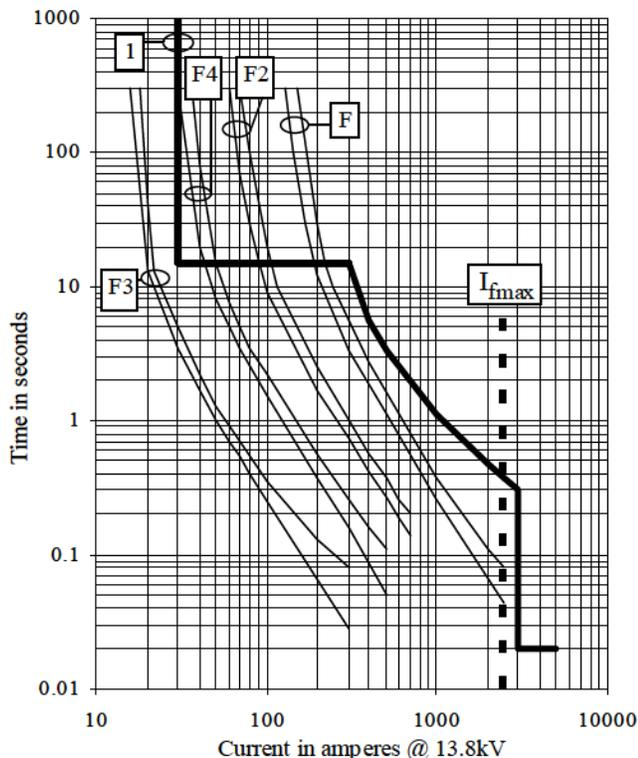
Fig. 12. Case of Fig. 3, considering 4 different downstream fuses, and the minimum melting current of one of them is similar to the pickup value of the nontraditional 51N function.
