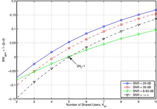
Fig. 3. Bandwidth gain of FBW compared to augmented code versus the number of shared users,  $K_{sh}$ .  $\alpha_{priv} = 10$  dB,  $\alpha_{sh} = 2$  dB,  $K = 6$ ,  $N_t = 3$ .
