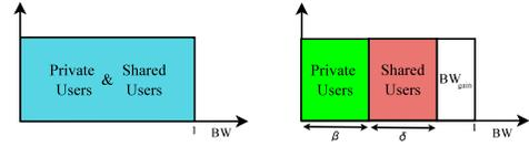
Fig. 2. Flexible Bandwidth scheme (FBW) compared to previous approaches.
