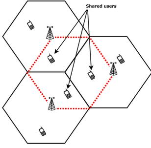
Fig. 1. 3-cell scenario with  $K = 1$  private user in each cell.  $K_{sh} = 3$  shared users are located within the edge area bounded by red dashed lines.
