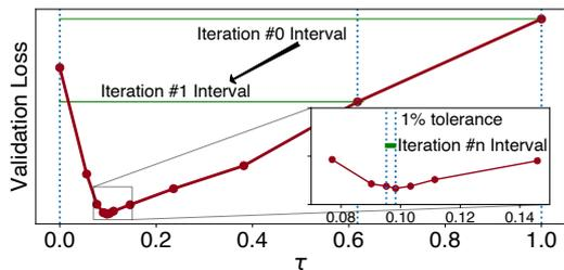
Fig. 2. Example of the sensitivity  $F(\tau)$  of the TES-RNN validation loss to the threshold  $\tau$  (here normalized by the traffic peak), in a practical forecasting task involving Snapchat traffic recorded at a network core datacenter. Dots denote the exploration steps of the Golden-Section search. The inset plot zooms onto the minimum loss, around which the final iterations of the algorithm occur.
