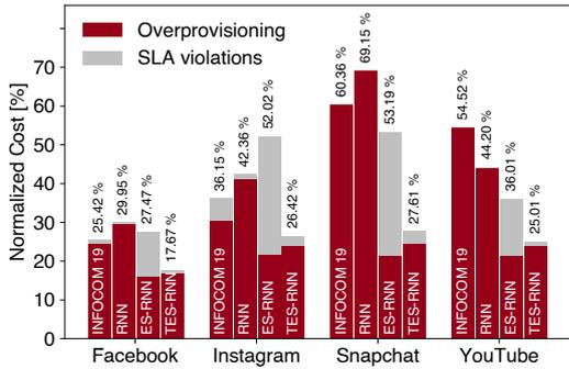
Fig. 5. Additional capacity allocation cost caused by INFOCOM19, RNN, ES-RNN, and TES-RNN prediction errors. Results refer to four slices assigned to specific services at a network core datacenter, with parameter  $\alpha = 3$ .
