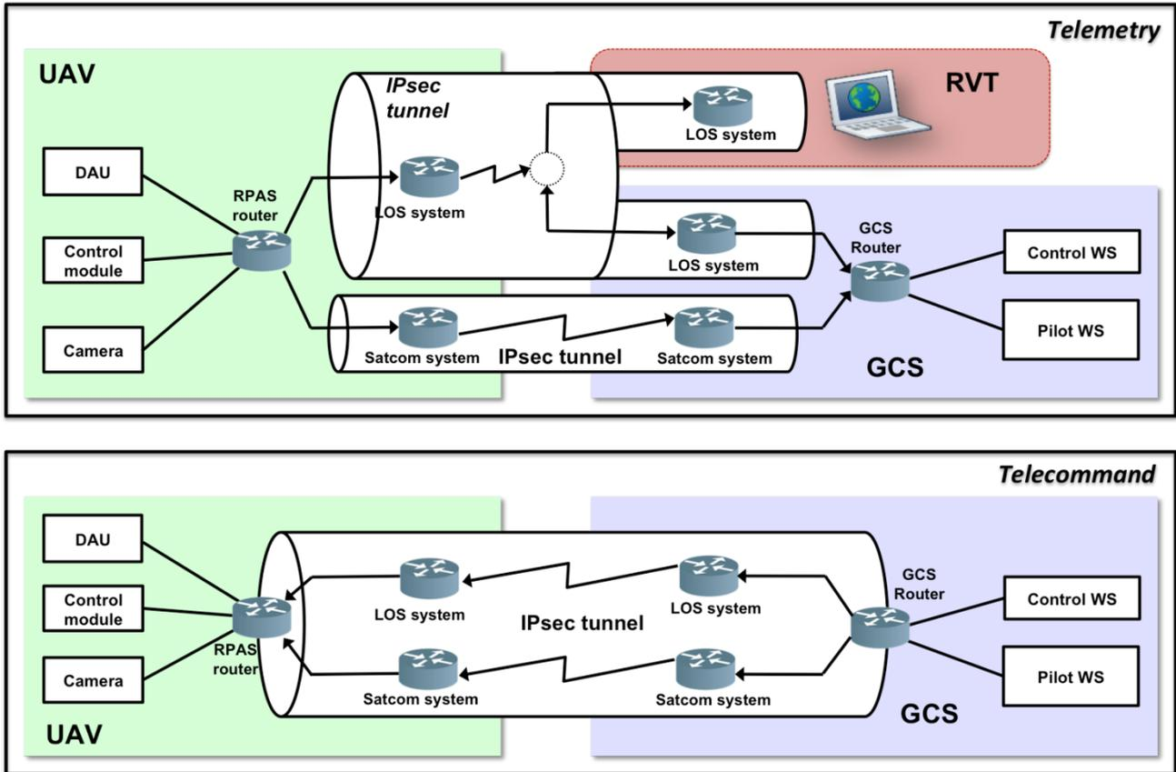
Figure 2: IPsec security for telemetry and tele-command
