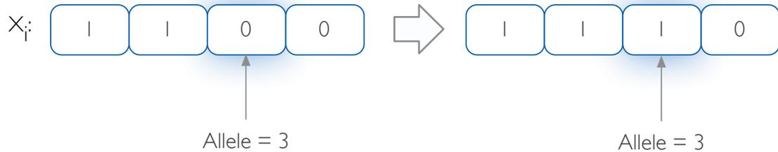
Figure 3.3: Mutation in genetic algorithms. A random value  $\chi$  is sampled anew for each allele in the binary string, if  $\chi \leq p_m$ , the allele value is inverted, otherwise, the bit value does not change.
