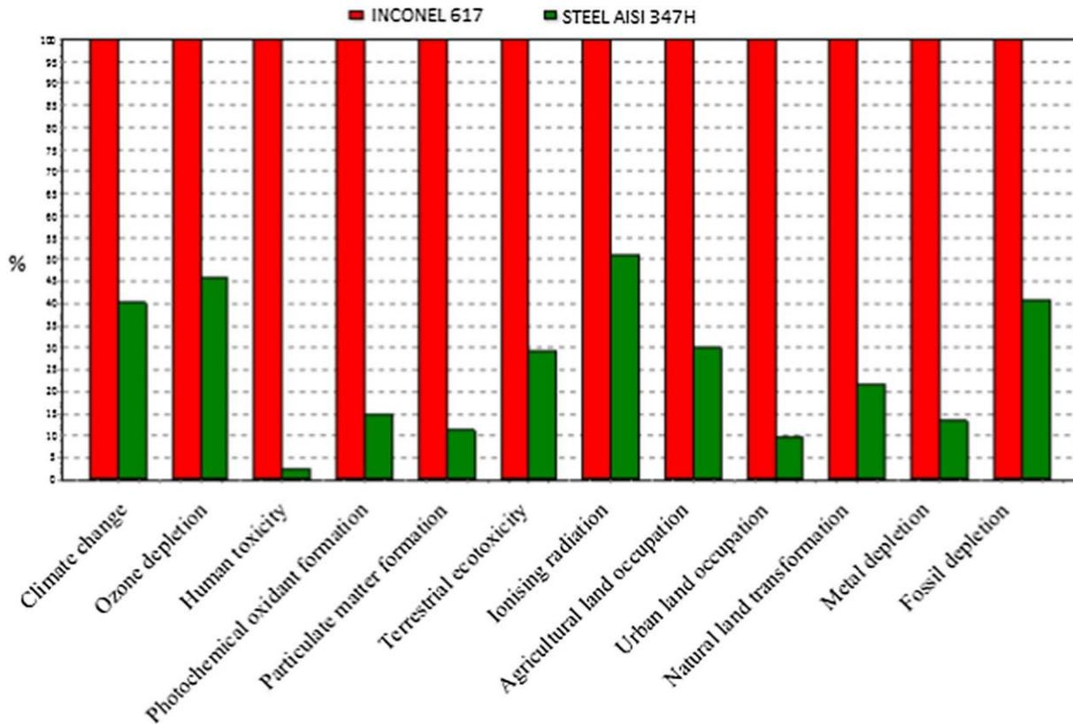
Fig. 6. Comparing 1 kg HRSA INCONEL 617 to 1 kg Stainless Steel AISI 347H; Method: ReCiPe Midpoint (H). Characterization. [% of environmental impact].
