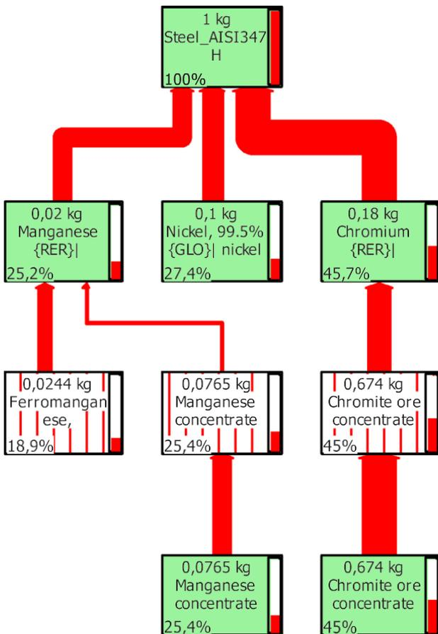
Fig. 3. Metal Depletion (kg Fe eq) impact category characterization network. AISI 347H stainless steel. ReCiPe Midpoint H. Cut-off value: 13%.
