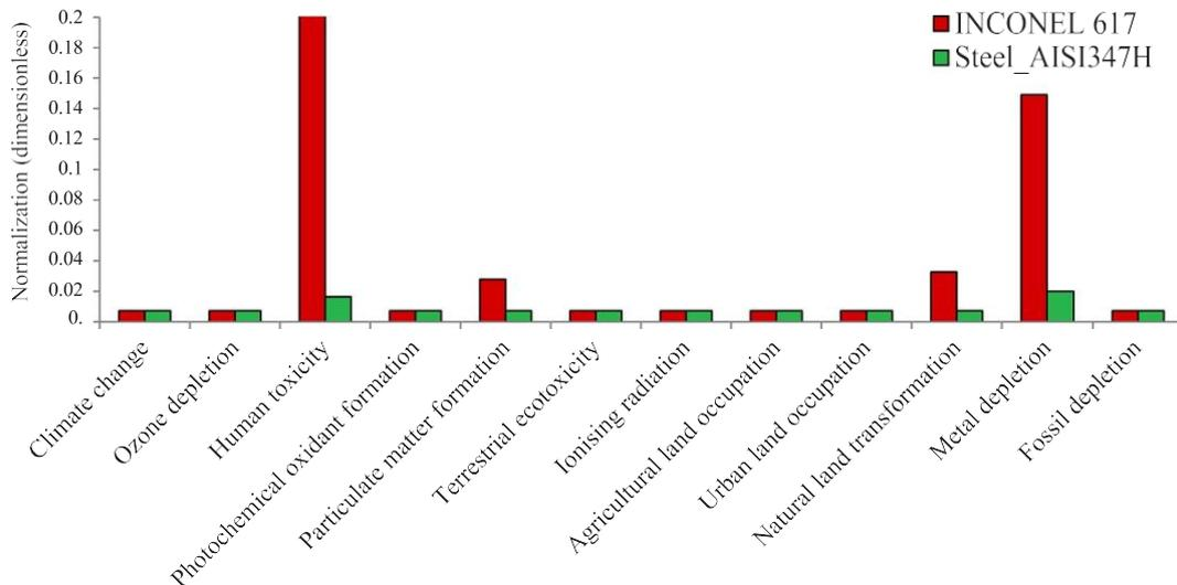
Fig. 7. Comparing 1 kg HRSA INCONEL 617 to 1 kg Stainless Steel AISI 347H; Method: ReCiPe Midpoint (H). Normalization. [dimensionless].
