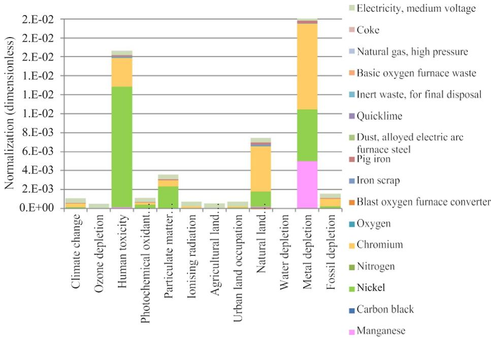
Fig. 2. Analyzing 1 kg AISI 347H steel; Method: ReCiPe Midpoint H. Normalization.
