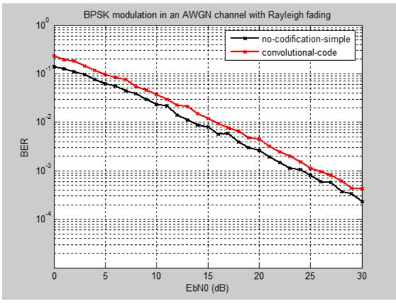
Figure 5.5: BPSK modulation in an AWGN channel with slow Rayleigh fading for blocks of length 100 bits
