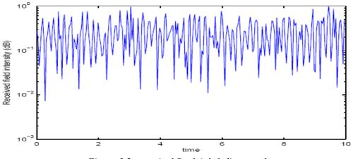
Figure 3.2: a typical Rayleigh fading envelope
