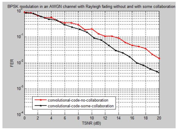
Figure 5.17: BPSK modulation in an AWGN channel with Rayleigh fading and some collaboration of the relay in the middle of source and destination, for blocks of length 260 bits
