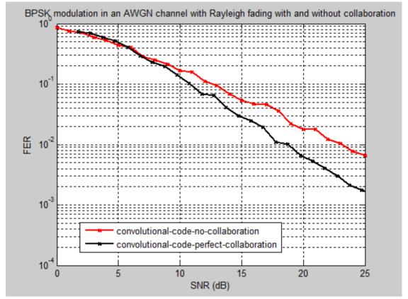
Figure 5.14: BPSK modulation in an AWGN channel with Rayleigh fading and collaboration of the relay near the source, for blocks of length 260 bits
