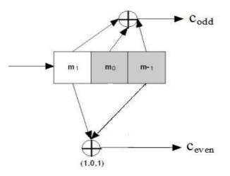
Figure 5.12: convolutional encoder for source and relay
