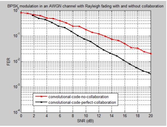
*Figure 5.16: BPSK modulation in an AWGN channel with Rayleigh fading and collaboration of the relay in the middle of source and destination, for blocks of length 260 bits*
