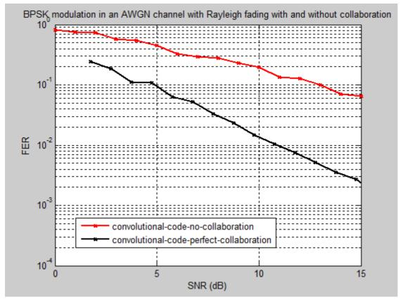
*Figure 5.15: BPSK modulation in an AWGN channel with Rayleigh fading and collaboration of the relay near the destination, for blocks of length 260 bits*
