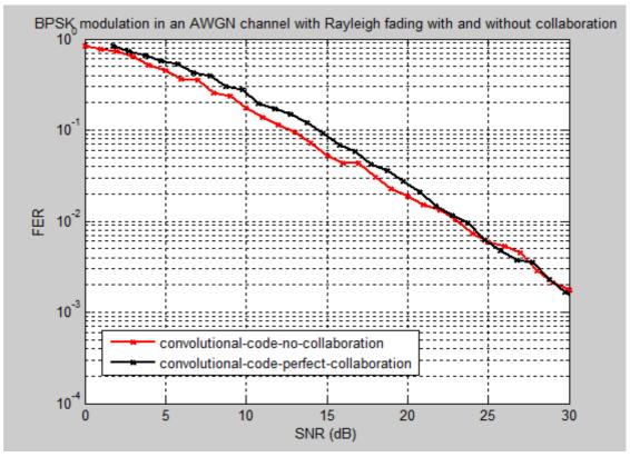
*Figure 5.13: BPSK modulation in an AWGN channel with Rayleigh fading and collaboration of the relay far from the source and the destination, for blocks of length 260 bits*
