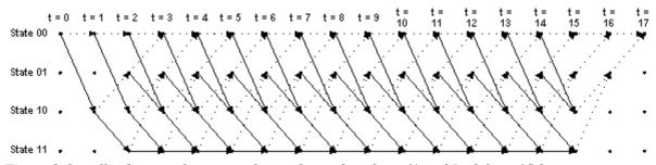
Figure 2.6: trellis diagram for a convolutional encoder of rate  $\frac{1}{2}$  and L=3 for a 15-bit message
