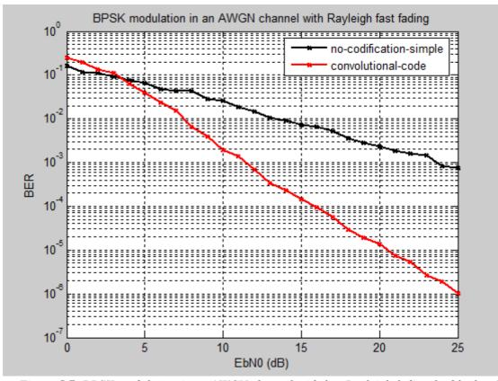
Figure 5.7: BPSK modulation in an AWGN channel with fast Rayleigh fading for blocks of length 10 bits
