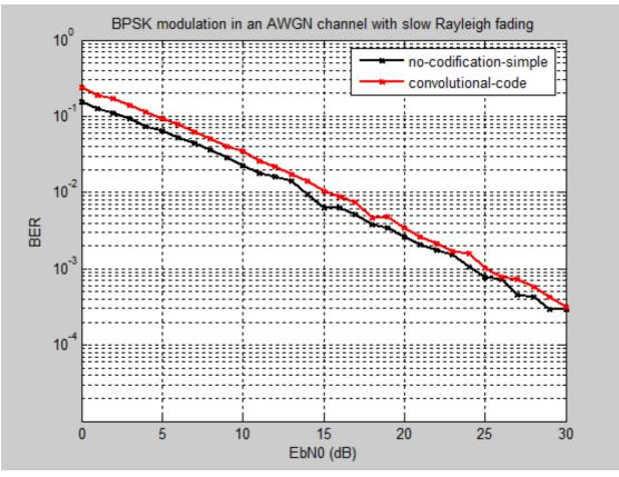
Figure 5.6: BPSK modulation in an AWGN channel with slow Rayleigh fading for blocks of length 1000 bits
