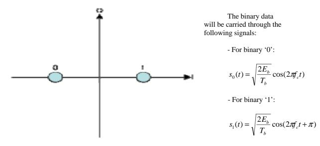
Figure 2.3: the constellation diagram for BPSK
