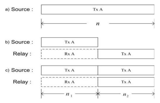
*Figure 4.3: a) direct transmission, b) collaboration with source silent in second phase, c) collaboration with source transmitting in the second phase*
