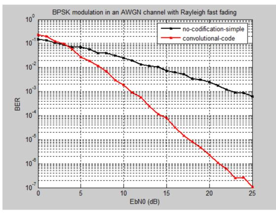
Figure 5.10: BPSK modulation in an AWGN channel with five different Rayleigh fading values for blocks of length 100 bits
