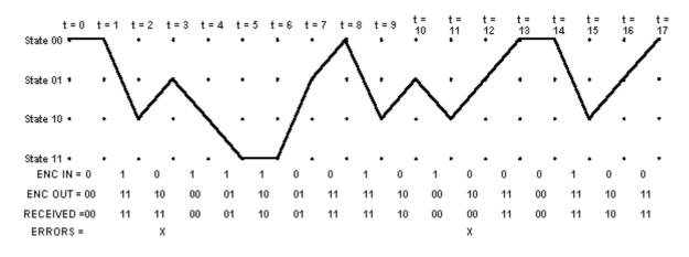
Figure 2.12: trellis optimum path after getting to the end
