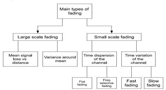
Figure 3.1: types of fading in radio channels
