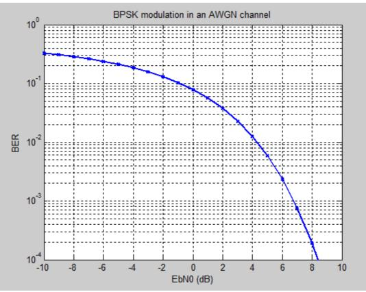
Figure 2.5: BER of BPSK modulation in AWGN channel
