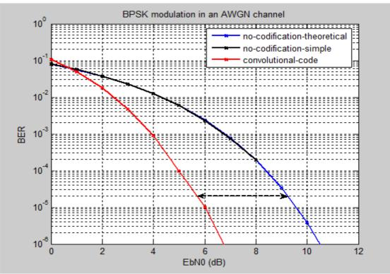
Figure 5.3: BPSK modulation in an AWGN channel for blocks of length 100 bits
