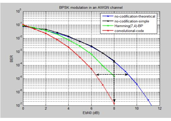
Figure 5.2: BPSK modulation in an AWGN channel for blocks of length 10 bits
