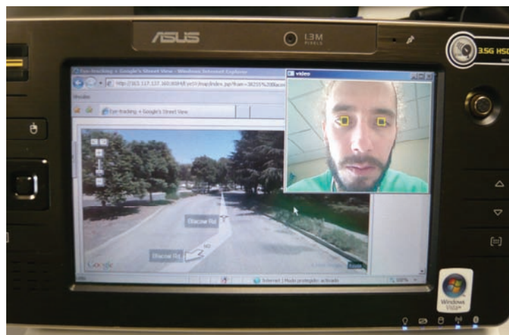
Fig. 5. The eye-tracker together with Google streetview running on an Ultra-Mobile PC equipped with wifi connection
