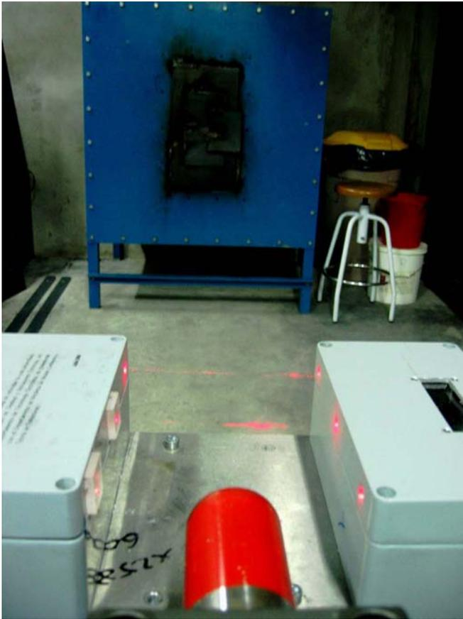
**Fig. 9** Photograph of the real system used for high-velocity impact testing of aircraft and spacecraft structures.
