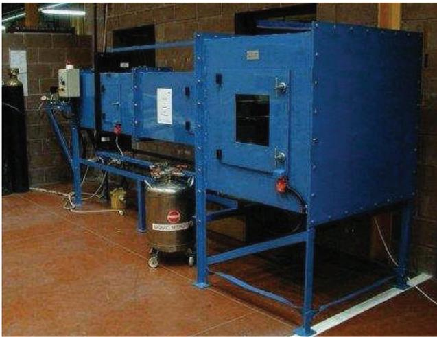
Fig. 9. Gas gun experimental device.
