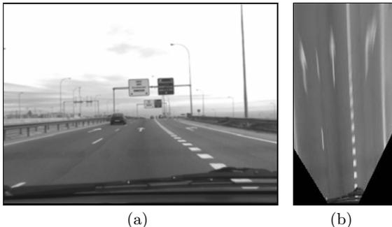
**Fig. 2.** (a) On-board camera-view; (b) Bird-eye view
