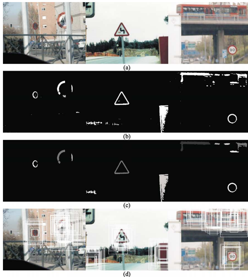
Fig. 5. Initialisation. (a) Original image; (b) thresholded image; (c) blob detection; (d) initial population location.
