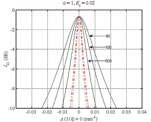
**Fig. 11.** The effect of  $N$  on BW. Solid lines: moderate SS type I mirror,  $n_3 = 0$ ,  $n_4 = 0.25$ ,  $N_C = 600$ , dash-dot lines: type II mirror,  $n_3 = 0$ ,  $n_4 = 0$ ,  $N_C = 736$ ,  $K_c = 0.02$ ,  $\alpha = 0$ . The parameter is the nominal mode number, the smaller the  $N$  the wider is the BW. Type II and type III mirror responses are virtually identical.
