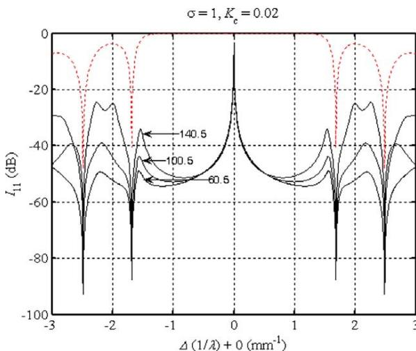
**Fig. 4.** Reflected intensity as a function of detuning for the type II mirror. The parameter is the mode number of the ring,  $n_3$  ( $n_4$ ) = 10 or 10.5, while the other parameters are the same as in Fig. 2. In the vicinity of  $K = 0.5$  the response is virtually independent of  $K$ . This characteristic also applies to type III mirrors, but with a different set of mode numbers (see Table 1).
