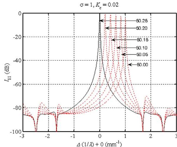
**Fig. 8.** The evolution of the reflected intensity spectrum in type I mirror. The parameter is  $N$ ,  $n_3 = n_4 = 10.25$ ,  $K = 0.4944$ ,  $\alpha = 0$ ,  $N_c = 600$ ,  $GS = 3.92$ . When  $N = 50$ ,  $\delta f \approx 1.28$  GHz for  $\delta N = 1 \times 10^{-3}$ .
