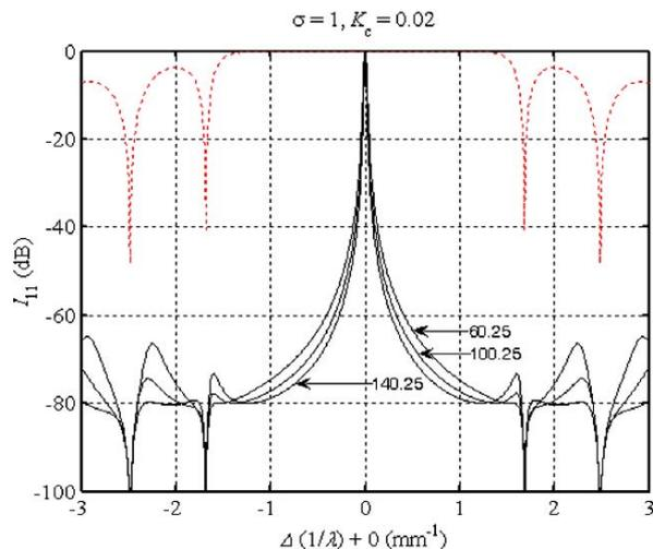
**Fig. 2.** Reflected intensity of the type I mirror for three mode numbers when  $n_3 = n_4 = 10.25$ . Also shown (dotted line) is the reflection loss characteristics of the gratings.  $N_G = 600$ ,  $n_a = 4.5294$ ,  $n_b = n_{\text{eff}} = 4.5$  ( $GS = 3.92$ ),  $K = 0.4944$ ,  $K_c = 0.02$ ,  $\lambda_0 = 1.5791 \mu\text{m}$  and  $\sigma = \exp(\alpha L)$ . Multiply the abscissa by  $3 \times 10^2$  to obtain the detuning in GHz. As  $|K - 0.5| \rightarrow 0$  the SS increases.
