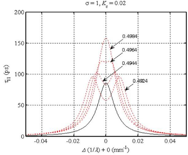
**Fig. 14.** Group delay in reflection of type I mirrors,  $\alpha = 0$ ,  $N = 100.25$ ,  $N_c = 600$  ( $GS = 3.92$ ),  $K_c = 0.02$ , the parameter is  $K$ . Dotted lines:  $n_3 = n_4 = 0.25$  (high SS), solid line:  $n_3 = 0.25$ ,  $n_4 = 0$  (same plot for all four  $K$  values).
