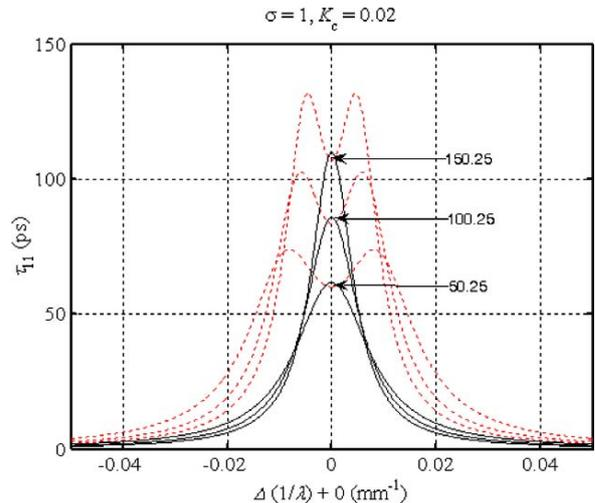
**Fig. 15.** Group delay in reflection of lossless type I mirrors. Solid curves: moderate SS ( $n_3 = 0.25$ ,  $n_4 = 0$ ), dotted curves: high SS ( $n_3 = n_4 = 0.25$ ). The parameter is  $N$ ,  $N_c = 600$  ( $GS = 3.92$ ),  $K_c = 0.02$ ,  $K = 0.4944$ .
