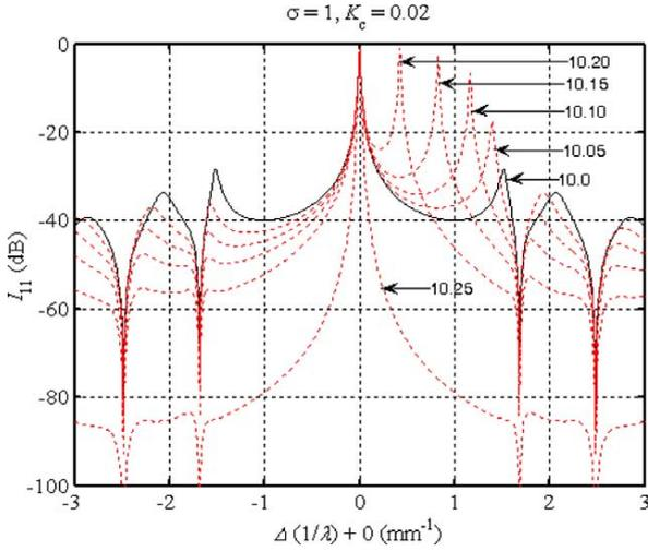
**Fig. 9.** Type I mirror. Morphing of low into high SS as  $n_3$  increases from 10 to 10.25.  $N = 50.25$ ,  $n_4 = 10.25$ ,  $K = 0.4944$ ,  $\alpha = 0$ ,  $N_C = 600$ ,  $GS = 3.92$ . Notice that the resonant peak at  $f_0$  remains fixed.
