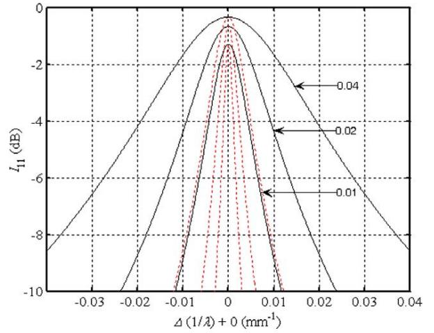
**Fig. 10.** The effect of  $K_c$  on BW. Solid lines: moderate SS type I mirror,  $N = 50.25$ ,  $n_3 = 0$ ,  $n_4 = 0.25$ ,  $N_C = 600$ ,  $\alpha = 0$ , dash-dot lines: type II mirror,  $N = 50.5$ ,  $n_3 = 0$ ,  $n_4 = 0$ ,  $N_C = 736$ ,  $\alpha = 0$ , (curves having the same maxima belong to the same  $K_c$ ). Characteristics for the type III mirror are virtually identical to those of the type II mirror.
