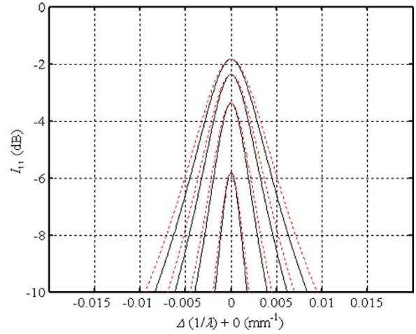
**Fig. 7.** Resonance peaks of lossless type II mirror. Solid lines:  $N = 140.5$ , dotted lines:  $N = 60.5$ ,  $n_3, n_4 = 10$  or  $10.5$ ,  $GS = 3.92$ ,  $K_c = 0.01, 0.02, 0.03, 0.04$ , the larger the  $K_c$  the smaller the RL and the wider the band. Very similar characteristics apply to type III mirrors with corresponding mode numbers.
