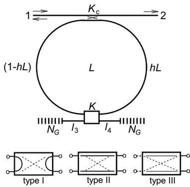
**Fig. 1.** Three types of grating-assisted microring resonator mirrors. The direct and coupled connections of the coupler  $K$ , detailed at the bottom, are indicated by the solid and dotted lines, respectively. The ring perimeter is  $L$ ,  $N_G$  is the number of periods in each grating, and  $h$  ( $0 < h < 1$ ) locates the coupler  $K$  on the ring. The attenuation coefficient of the waveguides is  $\alpha$ , the ring need not be circular.
