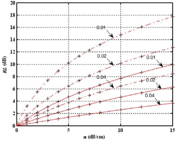
**Fig. 12.** Computed reflection loss at  $f_0$  in type I (solid lines) and type II (dash-dot lines) mirrors as a function of  $\alpha$ . The nominal mode numbers are:  $N = 100$ ,  $n_3 = n_4 = 0$ ,  $GS = 13$ ,  $K = 0.5$ . The parameter is  $K_c$ . The properties of the type III mirror are the same as those of the type II mirror.
