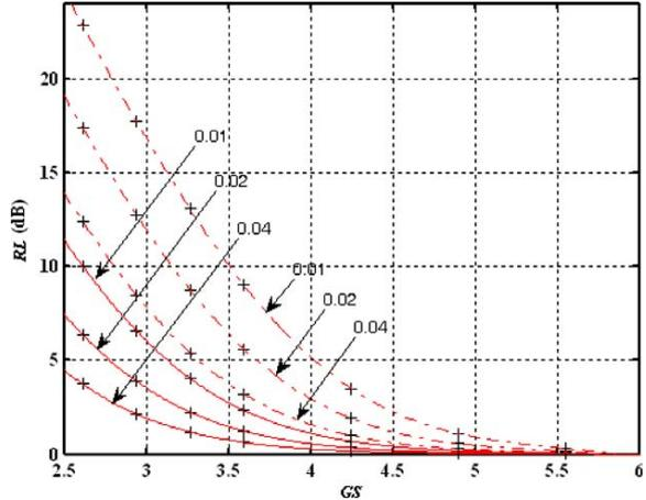
**Fig. 13.** Computed reflection loss at  $f_0$  in type I (solid lines) and type II (dash-dot lines) mirrors as a function of the GS. The nominal mode numbers are:  $N = 100$ ,  $n_3 = n_4 = 0$ ,  $\alpha = 0$ ,  $K = 0.5$ , the parameter is  $K_c$ . The characteristics of the type III mirror are the same as those of the type II mirror.
