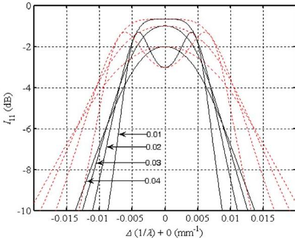
**Fig. 6.** Resonance peaks of lossless type I mirror. Solid lines:  $N = 140.25$ , dotted lines:  $N = 60.25$ ,  $n_3 = n_4 = 10.25$ ,  $GS = 3.92$ ,  $K_c$  is the parameter (solid and dotted plots with the same extrema correspond to the same  $K_c$ ).
