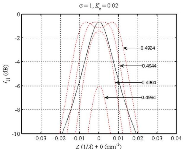
**Fig. 5.** Passband center of the lossless type I mirror for four values of  $K$ . Dotted lines:  $n_3 = n_4 = 10.25$ , solid line:  $n_3 = 10.25$ ,  $n_4 = 10$  (adjustment in  $K$  has no effect on the response).  $K_c = 0.02$ ,  $N = 60.25$ ,  $GS = 3.92$ .
