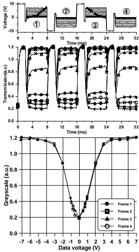
Fig. 6. Effect of saturation pulse on the transmission memory of the LC device.
