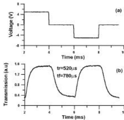
Fig. 3. (a) Voltage waveform and (b) optical transmission of the LC device in the time domain.
