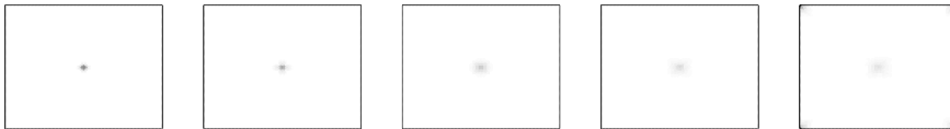
Figure 6: Absorption of a 0-investor for a pool of 1-investors with enough resistance to learning at time generations 10, 20, 100, 300, 1000 and 3000. B(x) = 4(1 - \exp(-x/2)) , C = 0.8 , \alpha = 0.65 . The asymptotic mean investment in the stationary state is almost 1.
