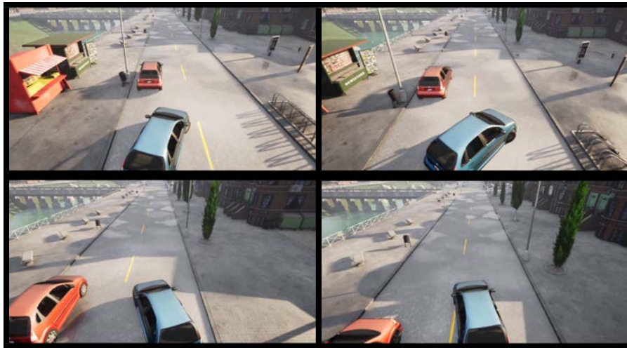
Fig. 5.18 CARLA frames from overtaking from the right side. The blue vehicle overtakes the red vehicle.
