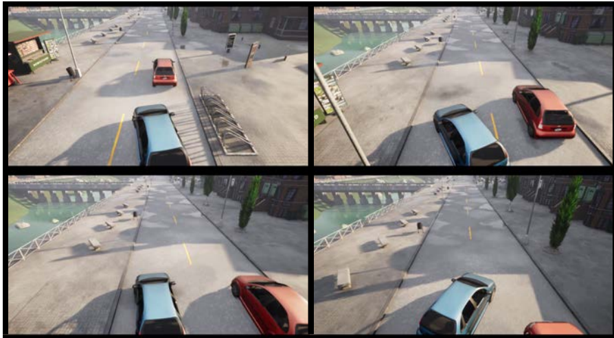
Fig. 5.15 CARLA frames from overtaking from the left side. The blue vehicle is the trained agent that overtakes the red vehicle.
