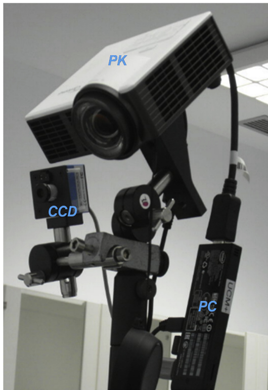
Fig. 8. Proposed light projection system , consisting of the Optoma® PK320 projector, that emits light onto of the painting, a DFK-72AUC02-F CCD camera, which was used to correct the spatial position of the system with respect to the illuminated printed picture, and the PC that processes the CCD data and applies the artificial vision algorithm to correct the image emitted by the projector according to the location of the printed picture.
