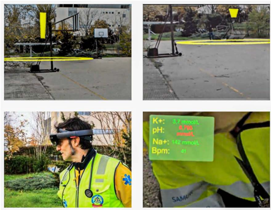
Figure 4.7: The object misplacement in the 4G without local edge scenario (top-left), a correct object placement in the 5G with local edge scenario (top-right), sanitary sta wearing the Hololens (bottom-left), patient health report shown on the Hololens (bottom-right).
