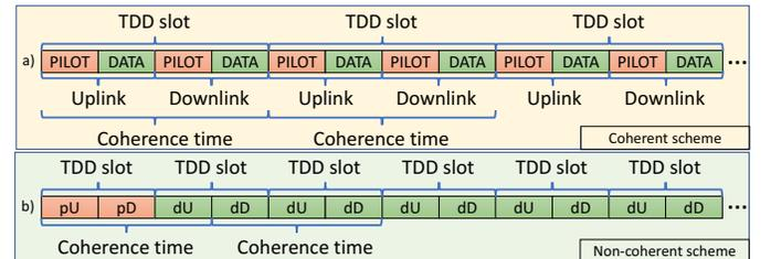
Fig. 1. TDD frame comparison for coherent (a) and non-coherent (b).
