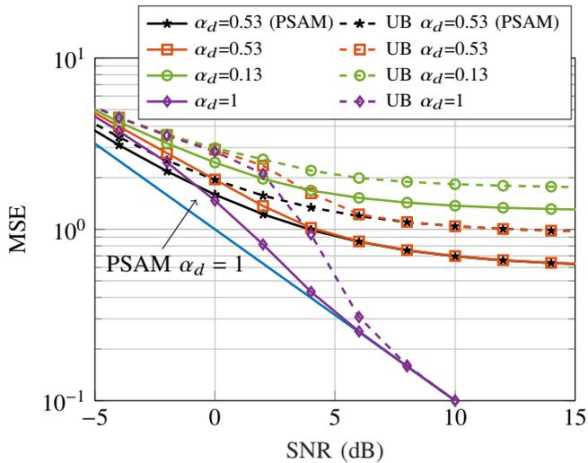
Fig. 2. MSE of channel estimation for  $M_{UL} = 16$  and  $R = 100$ . Continuous line corresponds to the Monte Carlo simulation while dashed line corresponds to the theoretical upper bound. Blue line represents the PSAM without channel time variability, which is the best case.
