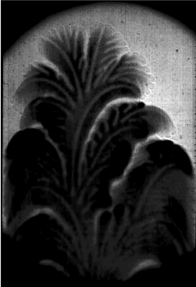
FIG. 2. Conventional continuous flame front structure.
