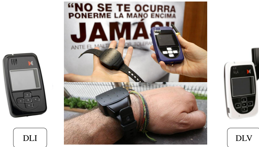
Figure 5-2: Devices considered for the electronic monitoring system within the "Protocol of action of the monitoring system by telematic means of the measures and sentences of restraint in matters of gender violence". DLI: Device worn by the aggressor; DLV: Device worn by the victim [7].
