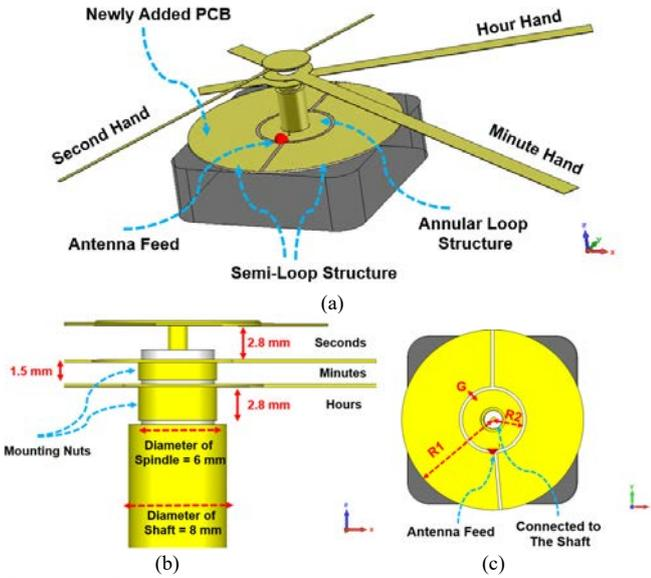
Fig. 3. (a) 3D view of the quartz clock with antenna feed using semi-loop and annular loop structures on a PCB. (b) Side view of the clock spindle and clock hands. (c) Top view of the PCB.
