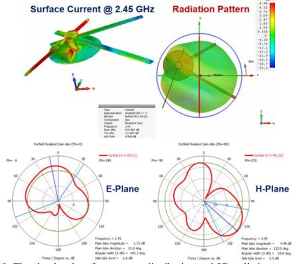
Fig. 8. The simulated surface current distribution and 3D radiation pattern of the clock antenna using 50 Ω port impedance and  $R_2 = 5$  mm at 2.45 GHz. The corresponding 2D patterns over the E-plane (elevation plane) and H-plane (azimuth plane) are shown as well.
