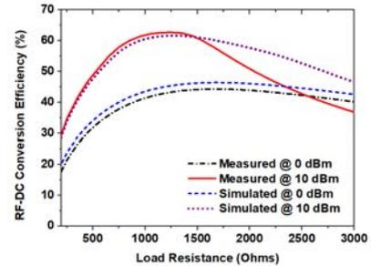
Fig. 16. The measured and simulated RF-DC conversion efficiency at two input powers vs. load resistance of the fabricated clock rectenna prototype. Note that the diodes are HSMS2850, chip capacitor is 100 nF, and frequency is 2.45 GHz.
