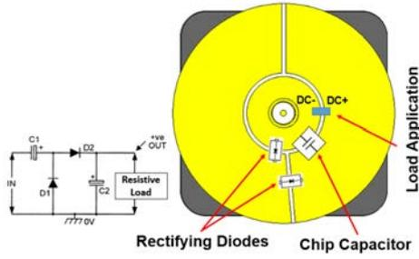
Fig. 9. Configuration of the simplified rectifier on the PCB and its equivalent circuit model.
