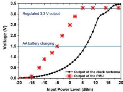
Fig. 18. Measured output voltage of the clock rectenna and the PMU vs. input RF power to the rectifier. The input voltage to the PMU is identical to the output voltage of the rectenna.
