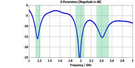
Fig. 5. Example of simulated reflection coefficient of the clock antenna for  $R_2 = 5$  mm and using 50  $\Omega$  port impedance.
