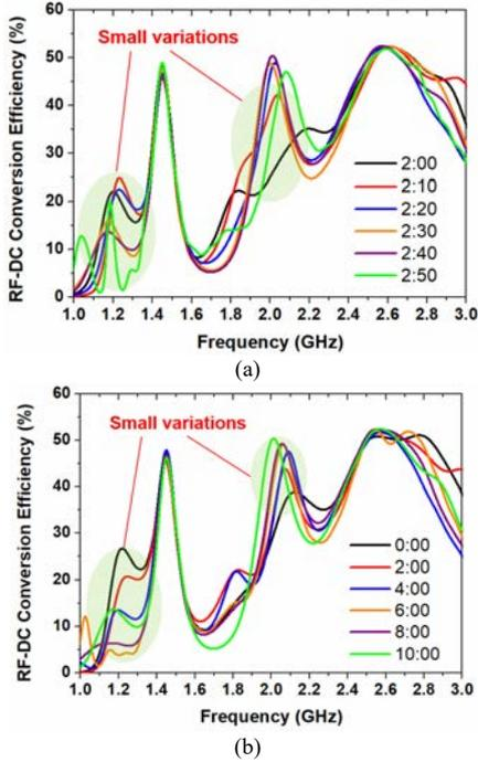
Fig. 12. The simulated RF-DC conversion efficiency of the complete clock rectenna ( $R_2 = 15$  mm) for (a) minute hand rotates from 2:00 to 2:50 and (b) hour hand rotates from 0:00 to 10:00. The input power is 0 dBm and load resistance is 1000  $\Omega$ .
