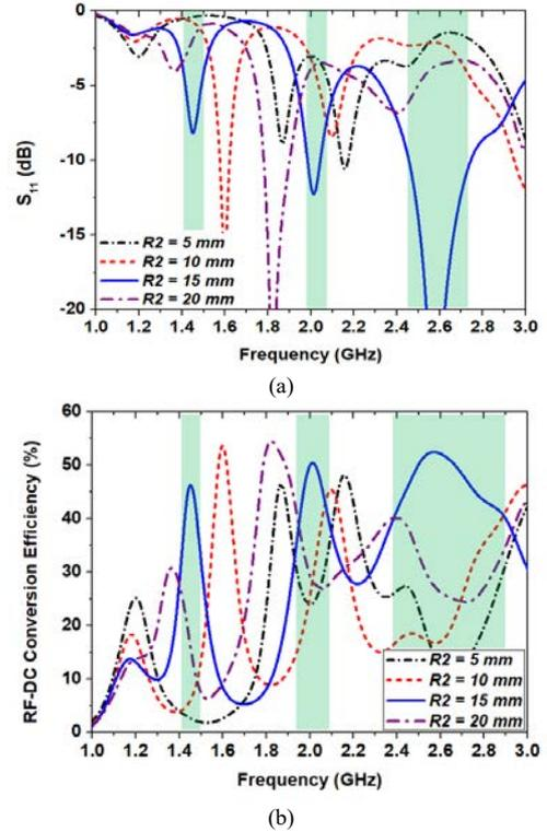
Fig. 10. The simulated (a) reflection coefficient and (b) RF-DC conversion efficiency of the complete clock rectenna. Note that the diodes are HSMS2850, chip capacitor is 100 nF, input power is 0 dBm and load resistance is 1000  $\Omega$ .
