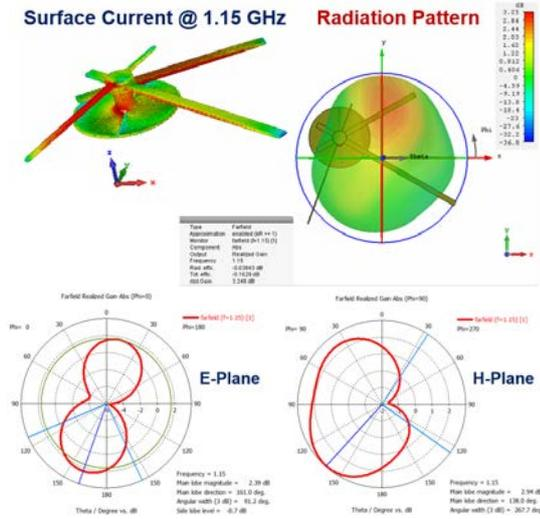
Fig. 6. The simulated surface current distribution and 3D radiation pattern of the clock antenna using 50 Ω port impedance and  $R_2 = 5$  mm at 1.15 GHz. The corresponding 2D patterns over the E-plane (elevation plane) and H-plane (azimuth plane) are shown as well.
