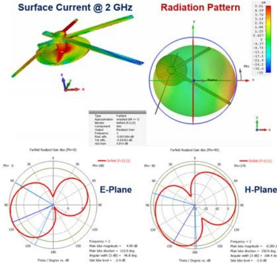
Fig. 7. The simulated surface current distribution and 3D radiation pattern of the clock antenna using 50 Ω port impedance and  $R_2 = 5$  mm at 2 GHz. The corresponding 2D patterns over the E-plane (elevation plane) and H-plane (azimuth plane) are shown as well.
