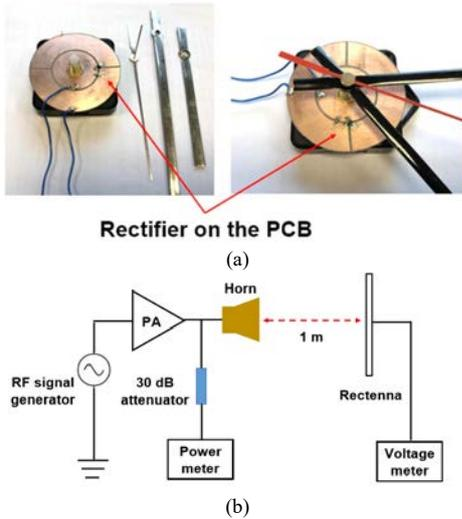
Fig. 13. (a) The fabricated clock rectenna example with and without the installation of clock hands. (b) Measurement setup of the clock rectenna. The rectenna orientation was tuned for the maximum output DC voltage during the measurement.
