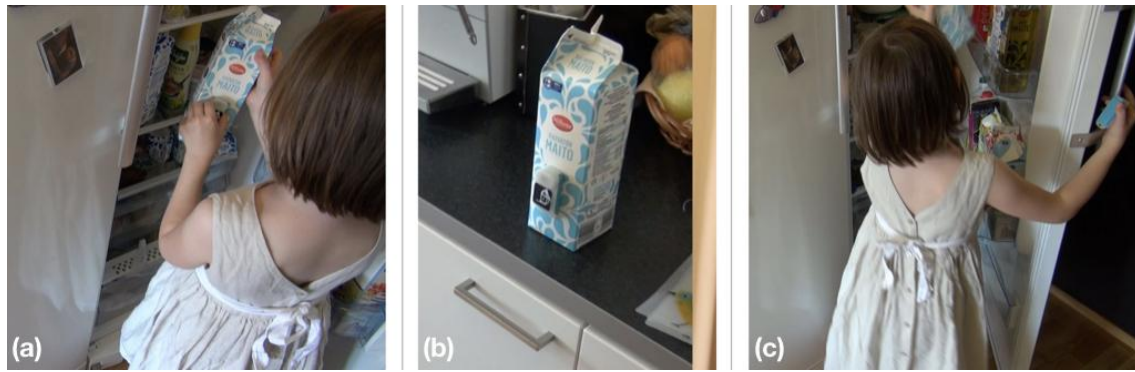
Figure 4: A sample scenario for the kitchen. (a) A token is attached to the milk box. (b) The token senses the milk box temperature when left on the kitchen counter and blinks or play a sound when it reaches 20 degrees. (c) Users are reminded to put the milk box back in the fridge.
