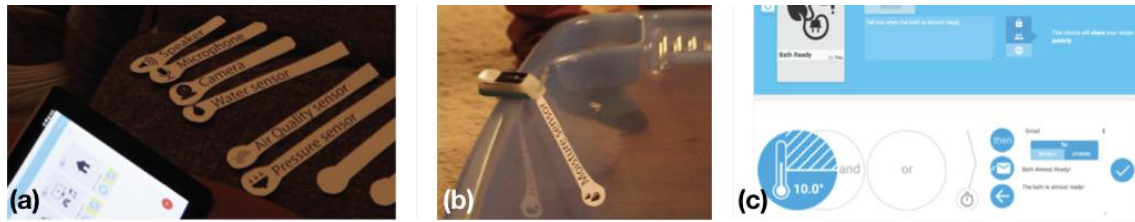
Figure 10: (a) Paper-based mockups of sensors and actuators that were provided to participants. They were also given blank mockups on which they could sketch desired technology. (b) Participants extended a token with a “water-level” sensor (they used the available mockup for a moisture sensor) and attached it to a bathtub for measuring the level of water while filling it. (c) Participants simulated the implementation of a recipe for such scenario: the “water-level” trigger was replaced with the available “temperature” trigger.
