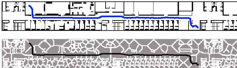
Figure 7: Trajectory calculated with Fast Marching over the Voronoi Diagram (Global map)
