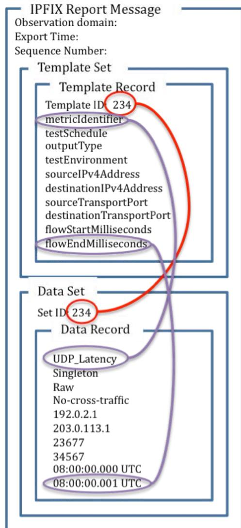
**Figure 4:** Example of an IPFIX report message for a UDP Latency test
