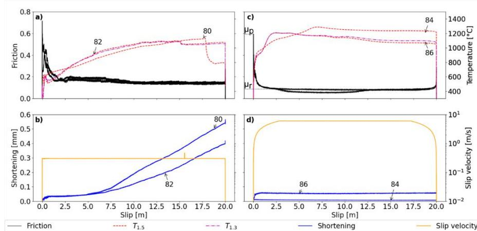
**Fig. 3.** Temperature increase measured with optical fibers in experiments performed on solid Carrara marble cylinders at a normal stress of 20 MPa. The Carrara marble was sheared at a target slip rate of  $0.3 \text{ m s}^{-1}$  (Figs. a and b) and  $3 \text{ m s}^{-1}$  (Figs. c and d) [Figure from 22].
