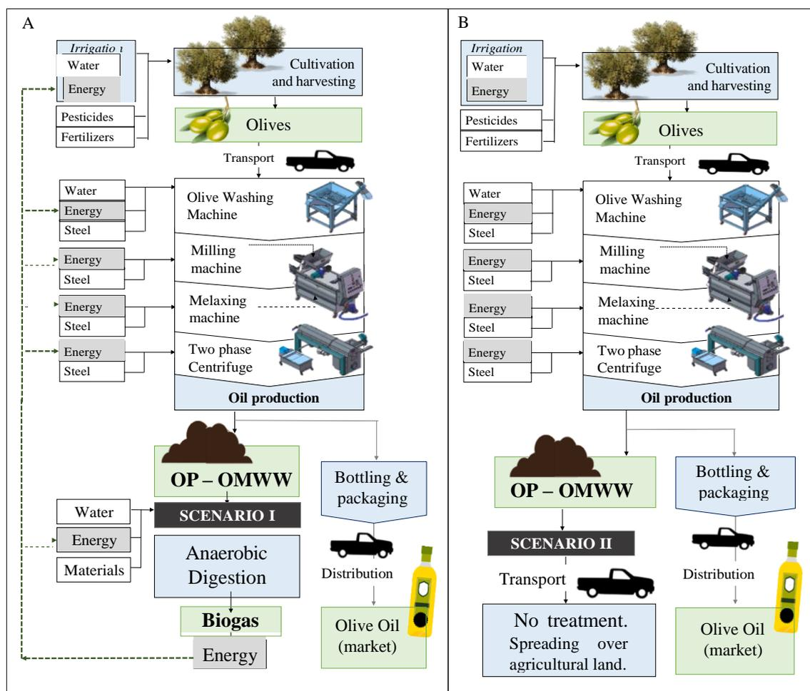
**Fig. 1.** Flowchart Diagram of the input and output in olive oil production system for 1 L of extra virgin olive-oil (EVO) and its waste treatment within the two examined scenarios. Part A and Part B represent scenario I and scenario II, respectively. Olive oil is only taken into account in terms of allocation.
