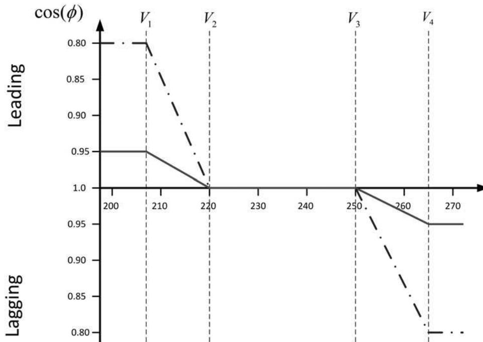
**Fig. 3** Power-factor control of draft AS/NZS4777.2
