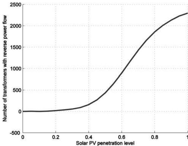
Fig. 5 Number of transformers with reverse power flow
