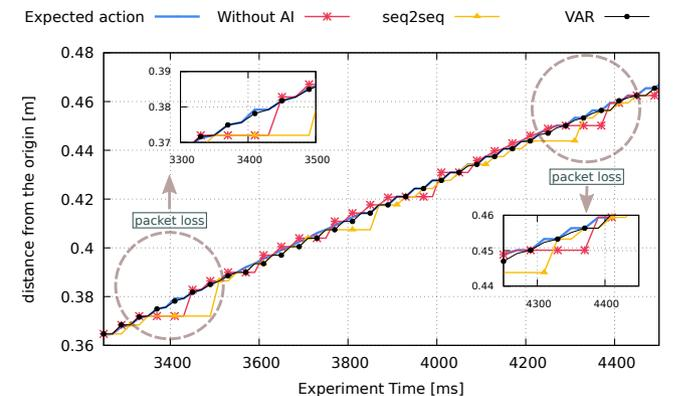
Fig. 4: Synchronization between Robotic Arm and Digital Replica
