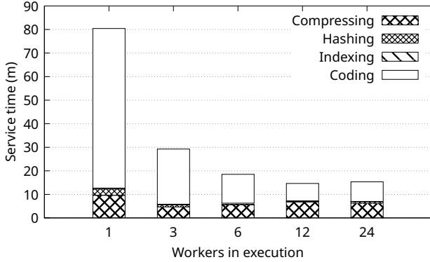
Fig. 7. Service time spent by the preparation scheme to process the DDSM dataset.
