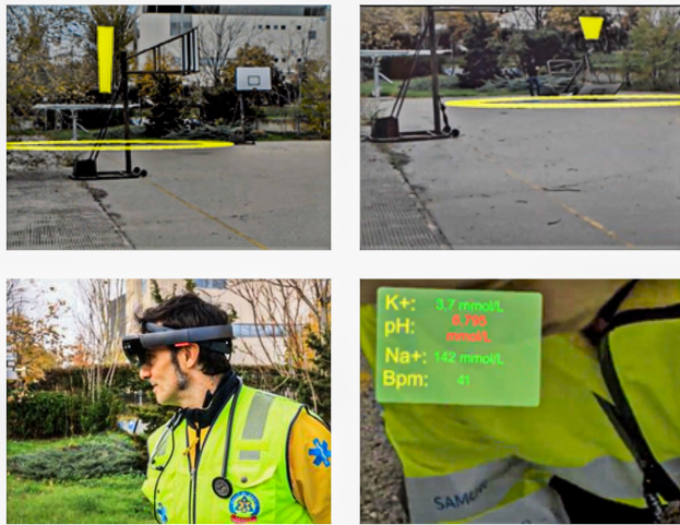
FIGURE 7. The object misplacement in the 4G without local edge scenario (top-left), a correct object placement in the 5G with local edge scenario (top-right), sanitary staff wearing the Hololens (bottom-left), patient health report shown on the Hololens (bottom-right).
