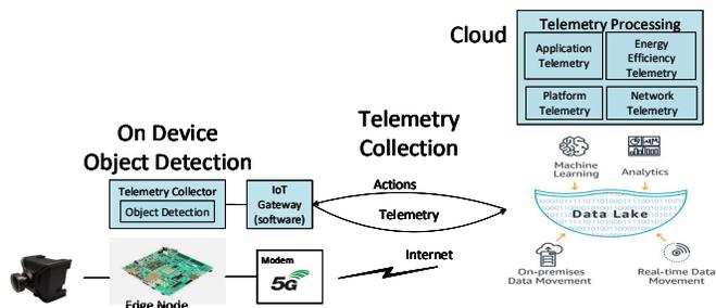
Fig. 1. Basic schematic of the telemetry framework
