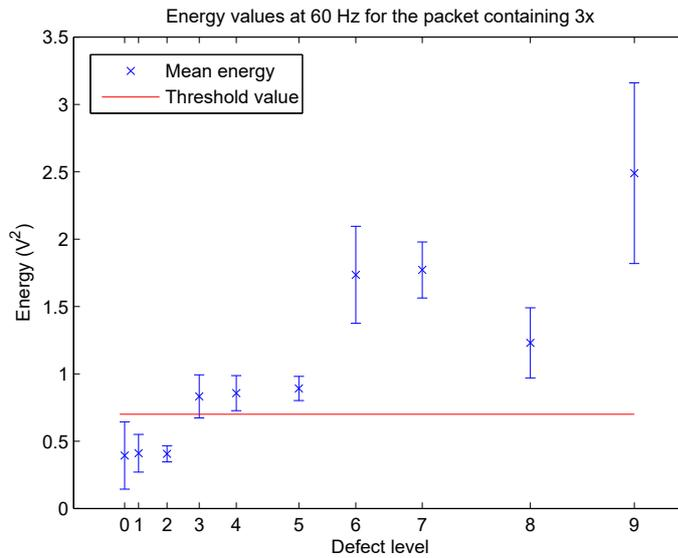
Fig. 10. Energy distributions in frequency bands related to 3x (represented by mean and standard deviation) versus the level of crack at 60 Hz
