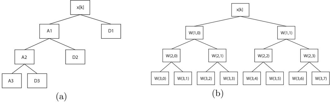
Fig. 3. Decomposition procedure for a signal  $x[k]$  to decomposition level 3 using (a) MRA analysis and (b) WPT analysis.
