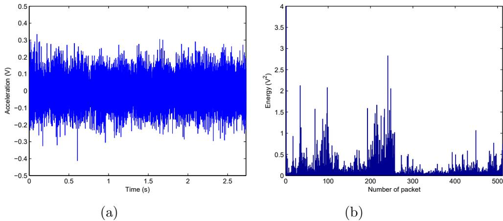
Fig. 4. Example of a WPT signal obtained for a healthy axle at 60 Hz showing (a) temporal signal and (b) WPT decomposition at level 9 (512 energy packets)
