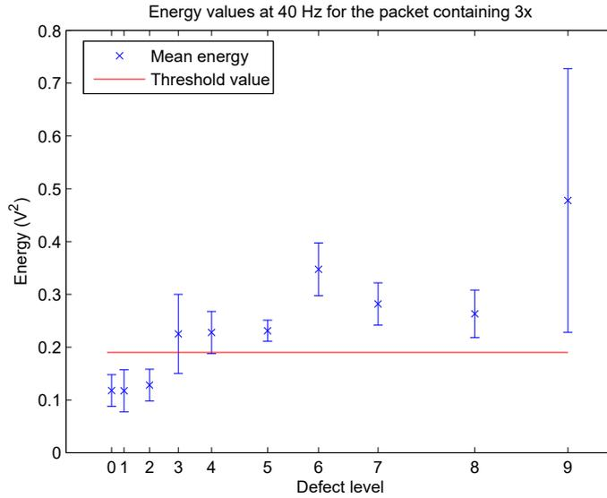
Fig. 9. Energy distributions in frequency bands related to 3x (represented by mean and standard deviation) versus the level of crack at 40 Hz
