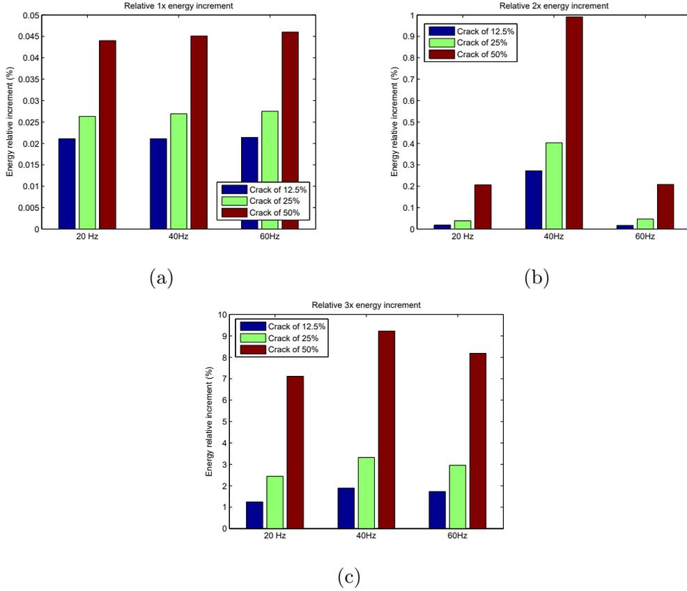
Fig. 7. Relative increments of energy regarding the healthy condition for the analytical model at different rotational speeds (Hz) found in packets related to (a) 1x frequency, (b) 2x frequency, and (c) 3x frequency.
