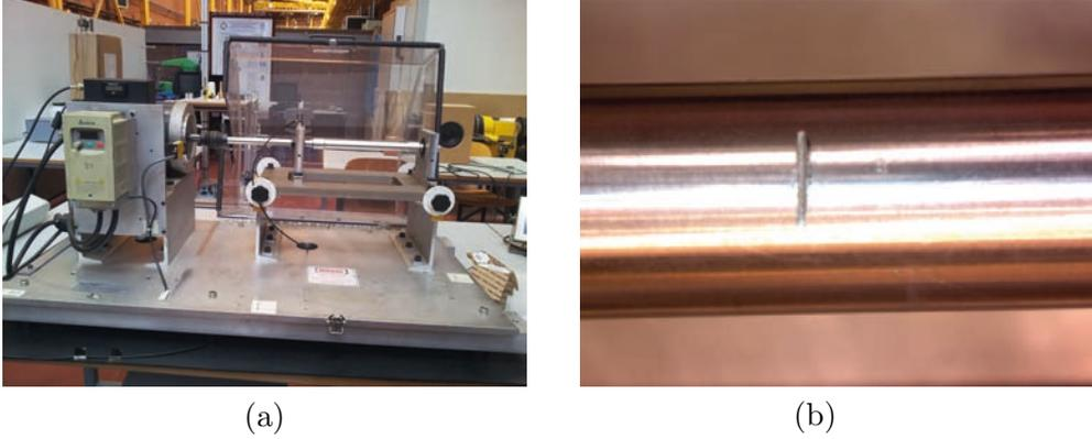
Fig. 2. Fault simulation rig (a) and detail of an induced defect (b).
