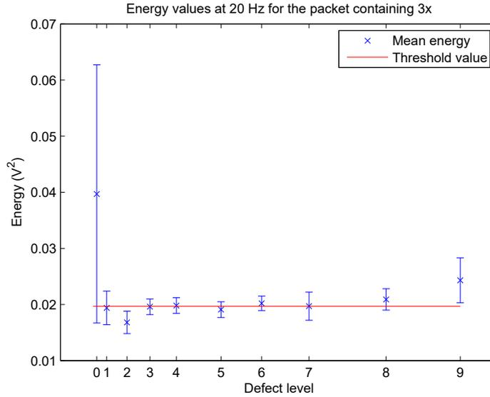
Fig. 8. Energy distributions in frequency bands related to 3x (represented by mean and standard deviation) versus the level of crack at 20 Hz.
