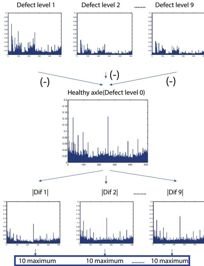
Fig. 5. Difference analysis procedure to detect increase in energy when a crack appears
