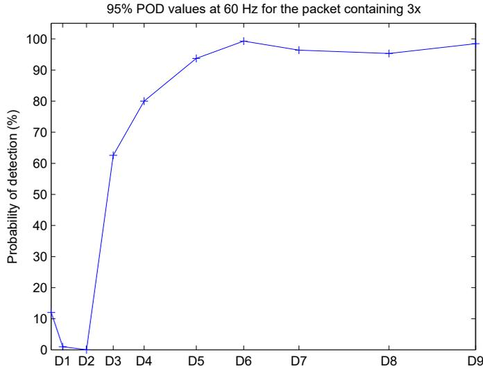
Fig. 12. POD curve at 60 Hz for the packet containing the 3x component at the 95% confidence lower limit.
