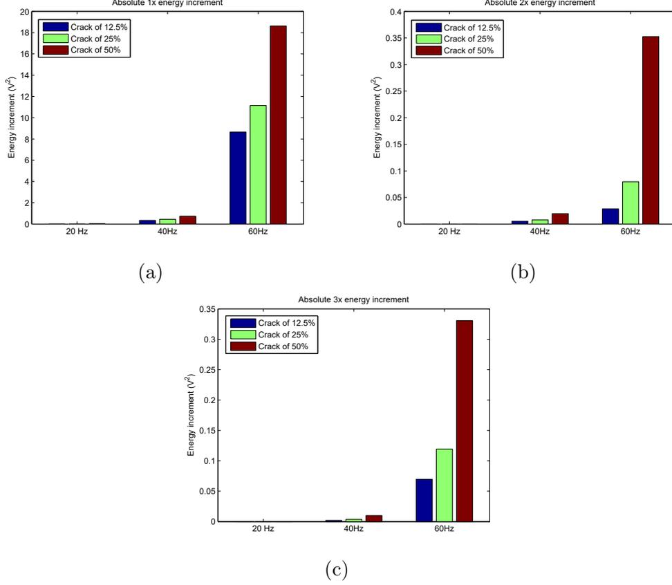
Fig. 6. Increments of energy regarding the healthy condition for the analytical model at the different rotational speeds (Hz) in packets related to (a) 1x frequency, (b) 2x frequency, and (c) 3x frequency.
