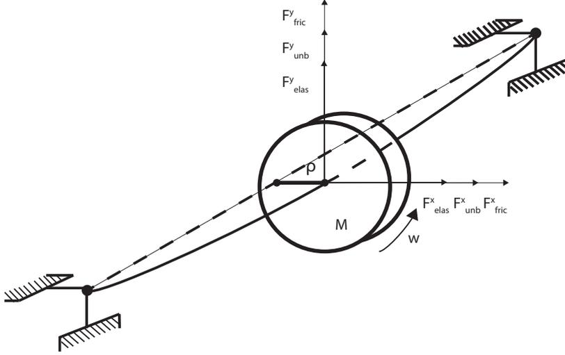
Fig. 1. Jeffcott rotor model and coordinate system.
