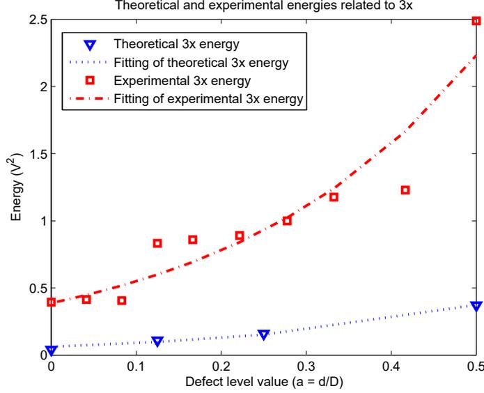
Fig. 11. Theoretical and experimental energies related to 3x at 60 Hz fitted to exponential functions.
