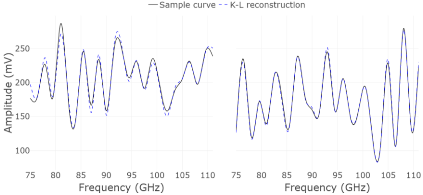
Figure 2-4. Two interpolated sample curves (black lines) with their corresponding K-L reconstruction using the first two principal components with an accumulative explained variance of 99.69%.
