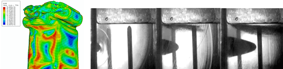
Left: Numerical simulation of the crash process resulting of the impact of an aluminium tube of a vehicle structure. Right: Impact sequence of the impact of a projectile onto an aluminium tank containing fluid (600 m/s).
