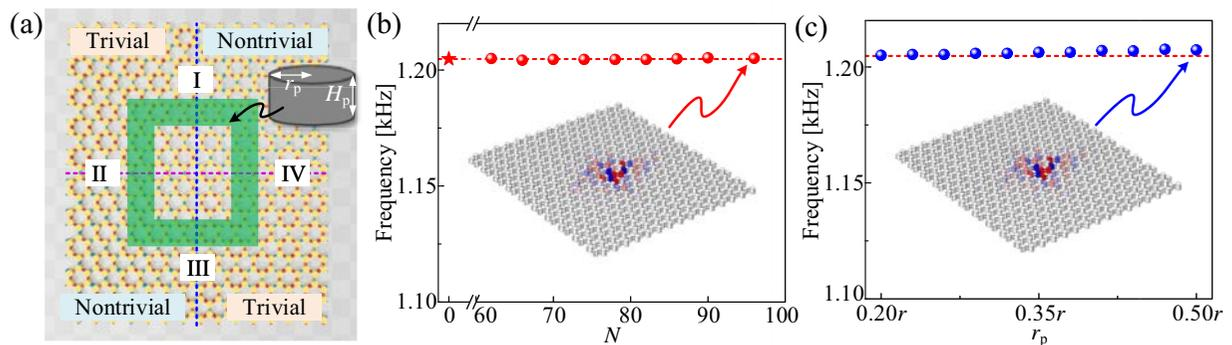
FIG. 5. (a) Within the shaded green (defect) zone, we introduce a number of rigid perturbation cylinders into the cavities where  $r_p$  and  $H_p$  are their radius and height. (b) Evolution of the corner states with the number of inserted cylinders  $N$ . (c) Same as (b), but here the radius of the perturbation cylinders  $r_p$  is increased. The red dashed line indicates the spectral location of the pristine corner state.
