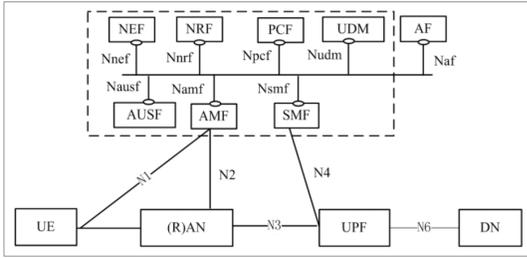
Fig. 3: 5G Service-based Architecture [21].
