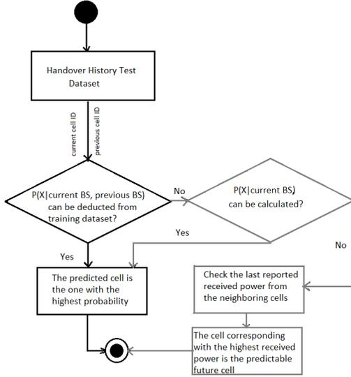
Fig. 2: Enhanced handover prediction algorithm workflow.
